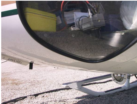
Figure 7. Digital video camera typical mounting location.
