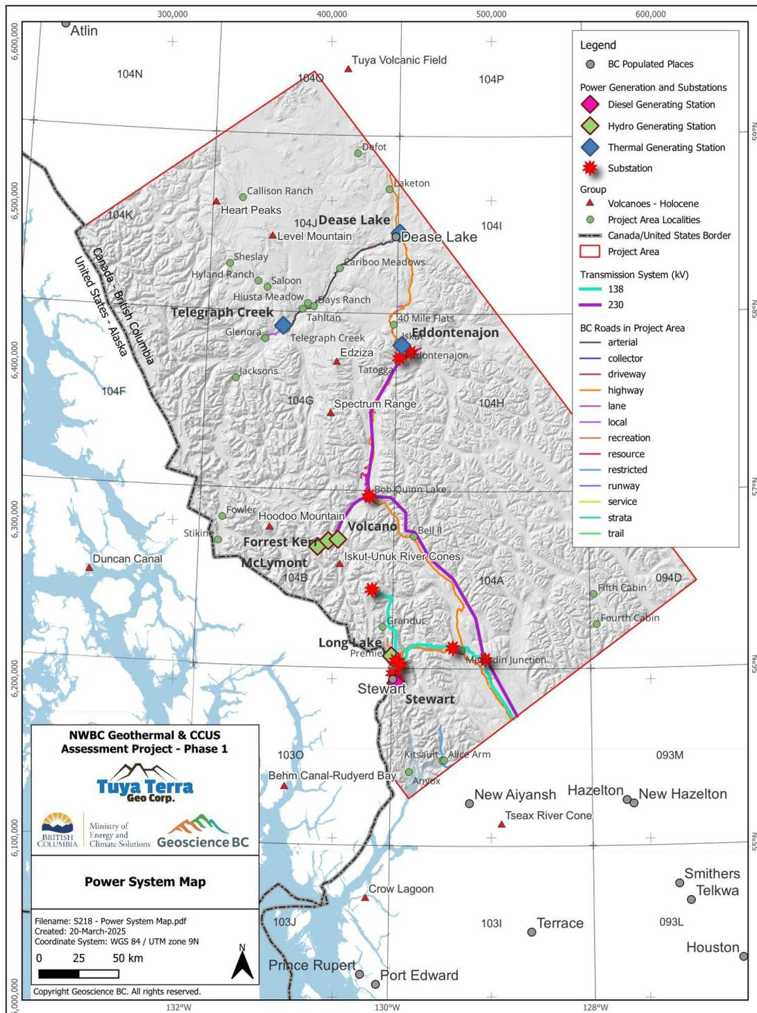
Section 2.18 Figure 3: Power System Map (transmission lines and power stations digitized from BC Hydro Transmission-System-2023-2024)
