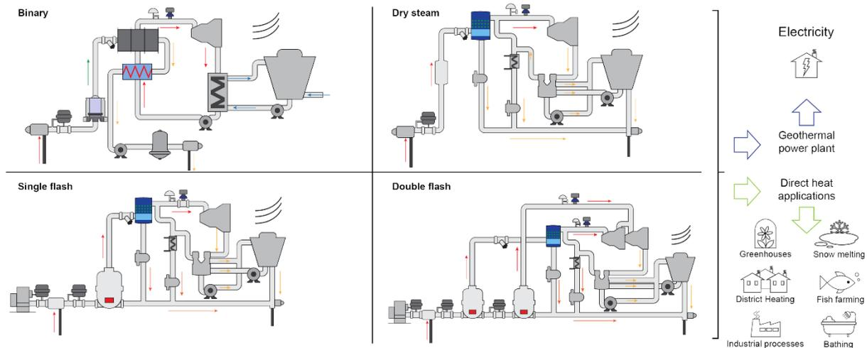
Section 1.1 Figure 3: Conventional geothermal systems (Class 2) use naturally occurring fluid (either liquid or steam) to create electrical energy. The type of system deployed is dependent on the specific characteristics of the resource as to temperature and liquid quality (i.e. dry or wet steam). (Moya et al., 2018, modified from their Figure 1)
