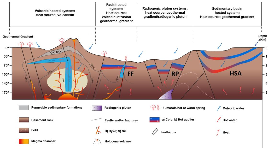
Section 1.1 Figure 2: Conventional geothermal systems (Class 2: Figure 1) form in a variety of geological settings: VH – volcanic hosted; FF – structural (fault and fractures); RP – radiogenic pluton; HSA – sedimentary basin. Depths and temperatures are approximate, based on a 34°C regional geothermal gradient. The gradient close to the volcano or intrusive dykes and sills, may be much higher as indicated by the 180°C isotherm. (Khodayar and Björnsson, 2024, modified from their Figure 1)
