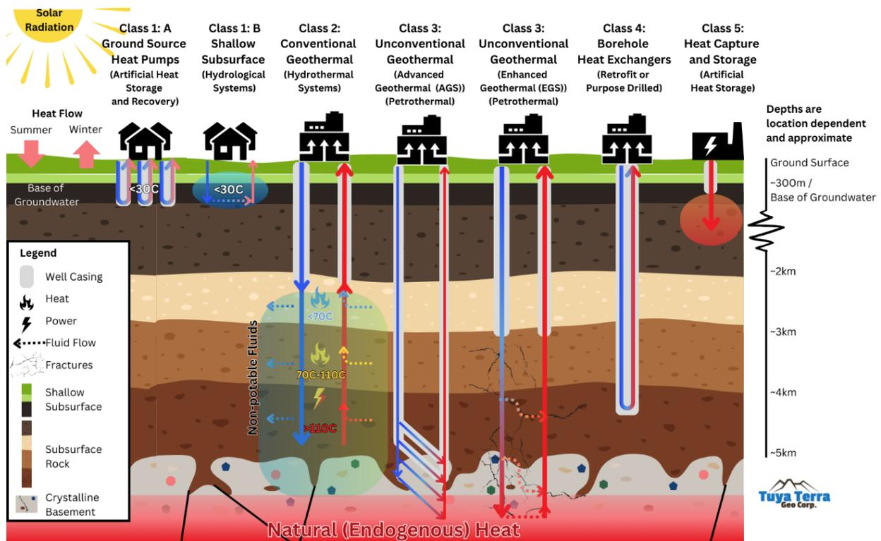
Section 1.1 Figure 1: Five classes of heat extraction (and storage) are shown in this schematic diagram first published in 2022 (Hickson and Smejkal, 2024). Class 2 systems are historically what make up the bulk of the global geothermal electrical generation.
