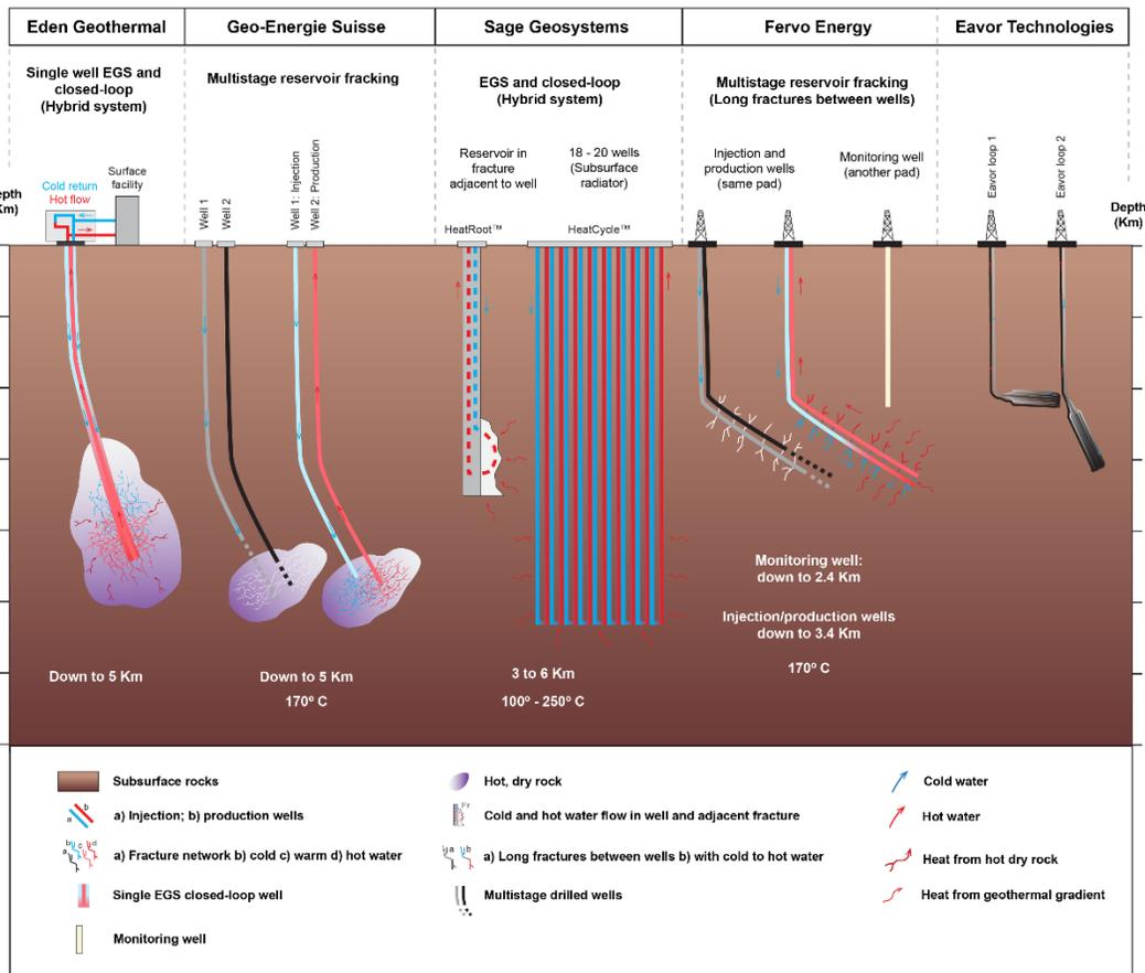
*Section 1.1 Figure 5: Unconventional geothermal developments: Enhanced or Engineered Geothermal Systems (EGS) in hot dry rock between 3 Km and 6 Km depth. EGS technology uses mostly hydraulic fracking to create fractures as natural heat exchangers in rock or adjacent to the borehole. AGS systems rely on a large surface area from many wellbores or groups of wellbores (a subsurface radiator) to extract thermal energy (Khodayar and Björnsson, 2024, modified from their Figure 4)*
