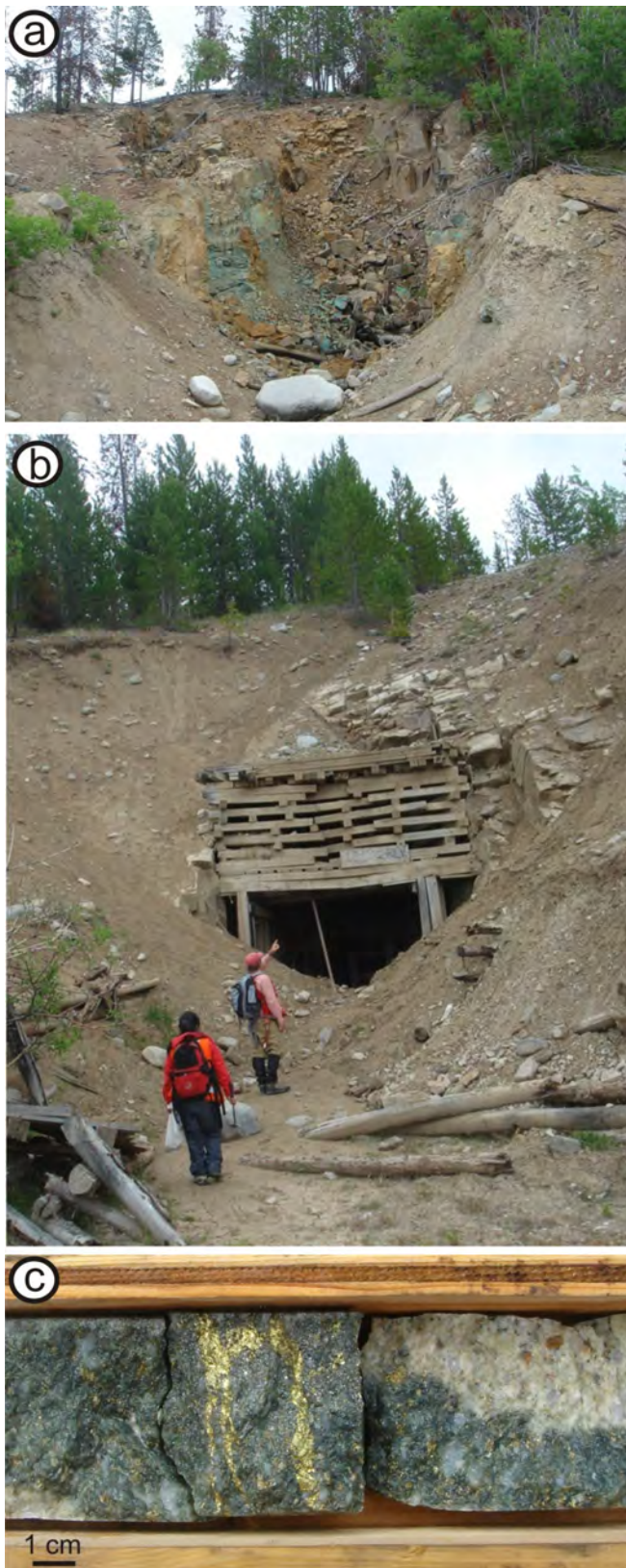
Figure 5: Highland Valley, Alwin mine: (a) Typical narrow, near vertical ore zone trending N70°E, oxidized at the surface. (b) Entrance of one of the old adits. (c) Example of very strong green muscovite alteration and associated chalcopyrite mineralization cutting the host Bethsaida granodiorite (AM-08-04A).
