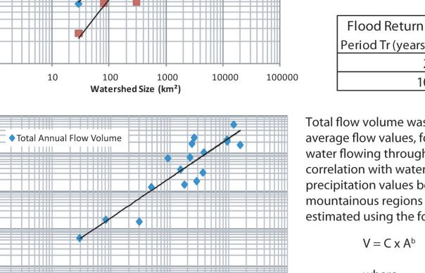
otal flow volume was calculated on a median annual basis using monthly average flow values, for stations with whole year records. Total volume of water flowing through drainages in the study area has a moderate to strong correlation with watershed size. Variation exists due to large differences in orecipitation values between some of the watersheds moving from more estimated using the following equation:  $V = C \times A^b$
