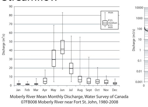
Hydrometric stations operated by the Water Survey of Canada were analyzed to identify several key parameters of flow characteristics in the study are
