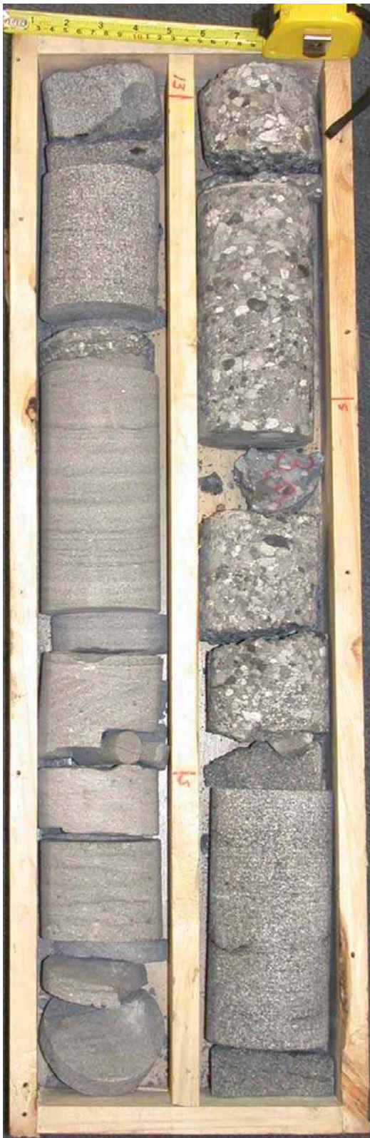
Lower Gething Formation. Interbedded poorly-sorted pebbly sandstone and better-sorted medium-grained lithic sandstone, exhibiting poorly-developed trough cross-stratification. (Top of core is to the upper right in the box) Numac North Red 15-1-86-22W6; 1212.2-1213.7 m.
