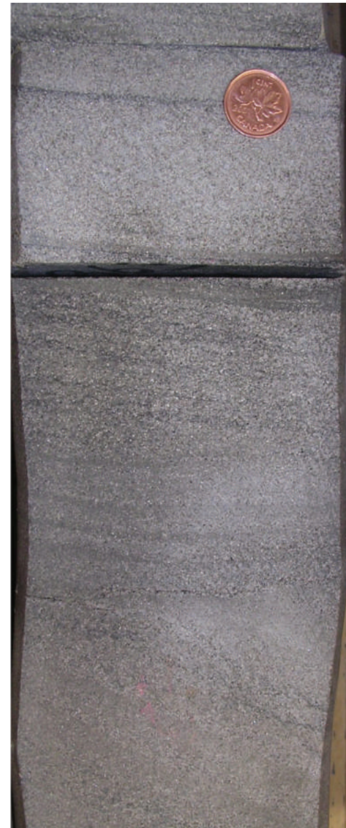
Laminated medium-grained shoreface sandstone in Halfway Formation at Blueberry. White "specks" are leached lithic sand grains, yielding limited secondary solution porosity. b-44-D/94-A-13, 1655.9 m
