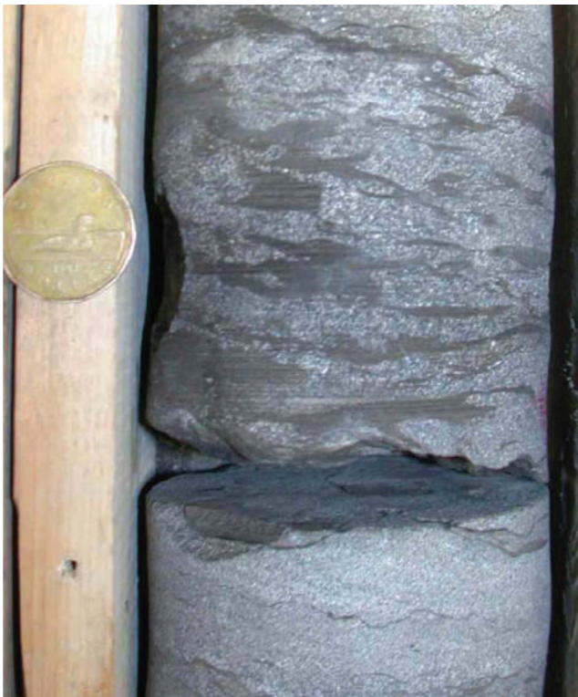
Buick Creek sandstone. Thin, flat, brown-grey mud clasts within massive Buick sandstone, interpreted as rip-up clasts transported only a short distance. Pacific East Siphon 6-4-87-15W6; 3668.5 ft.
