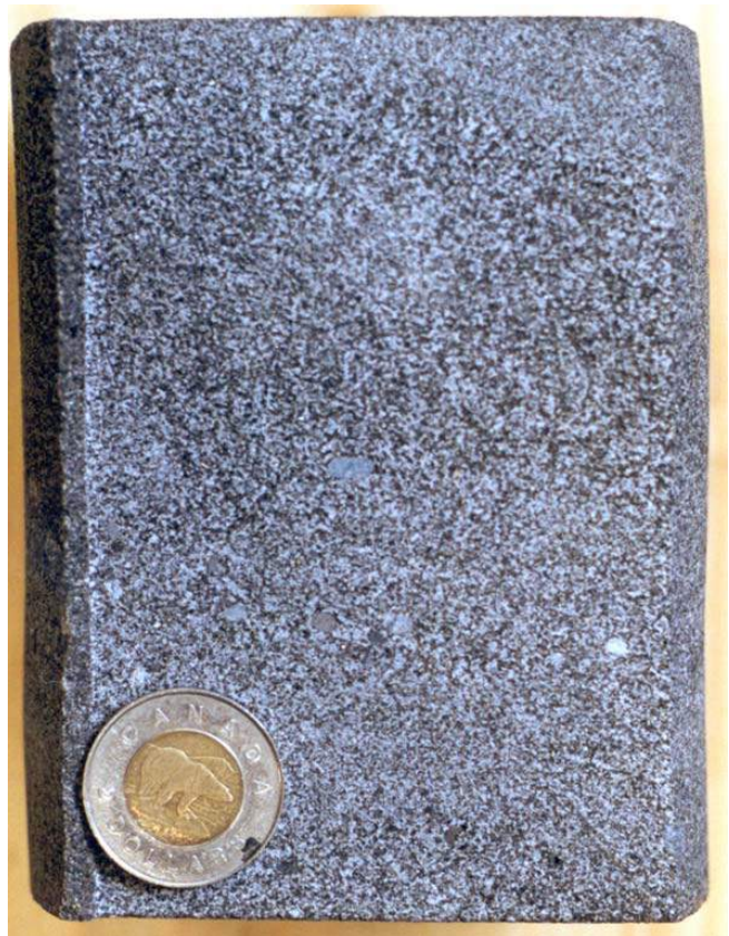
Lower Gething Formation. Massive, relatively well-sorted, medium- to coarse-grained lithic sandstone with good apparent porosity. Total Squirrel 10-4-88-19W6; 1194 m.
