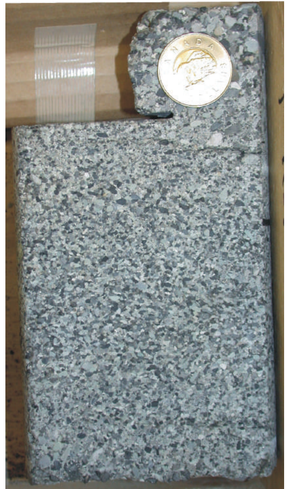
Well-sorted very coarse-grained sandstones to granule conglomerate of Cadotte foreshore, exhibiting good intergranular porosity. b-24-A/93-P-7, 2054.5 m.
