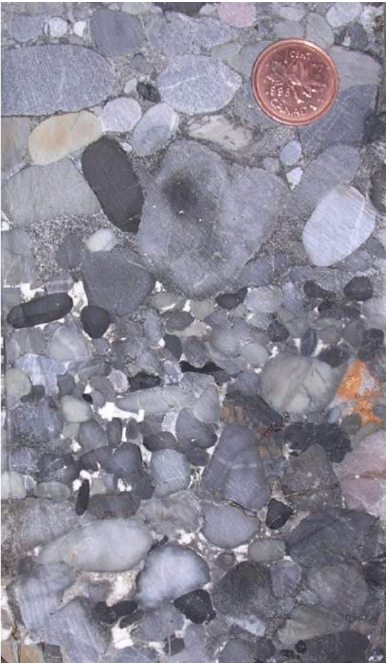
White (kaolinitic) clays fill isopated patches of interpebble porosity in a better-sorted interval. b-28-1/93-1-16; 2923 m.
