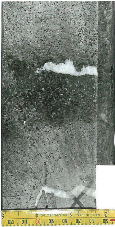
Core: leached pellet skeletal grainstone with moldic vuggy porosity after pellets and skeletal particles in fine crystalline dolomite with some intercrystalline porosity. White calcite vug and fracture fill. Slight oil stain. 7144 ft.
