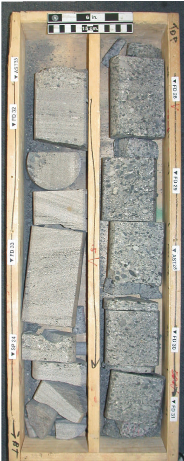
Cadotte upper shoreface, grading from cross-bedded pebbly sandstone up to sandy conglomerate. Sharp contact with finer-grained lower shoreface sandstones is near base of this interval, just below SP34 label. b-24-A/93-P-7, 2057.8 m.
