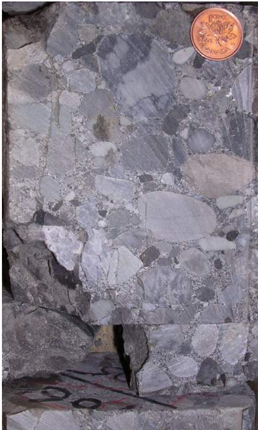
Close-up of fractured Cadomin conglomerate, illustrating pervasive sand filling interpebble porosity, with numerous short fractures breaking up several pebbles. b-28-1/93-1-16; 2919.6 m.
