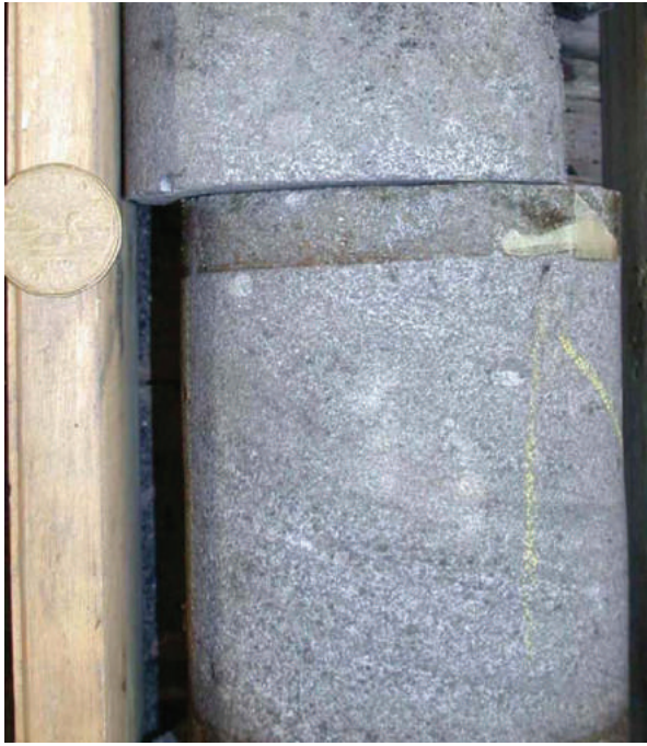
Buick Creek sandstone. Coarse-grained quartzarenite, exhibiting vague large-scale bedding interpreted as trough cross-bedding. Diasham West Stoddart 6-6-87-20W6; 1205.5 m.
