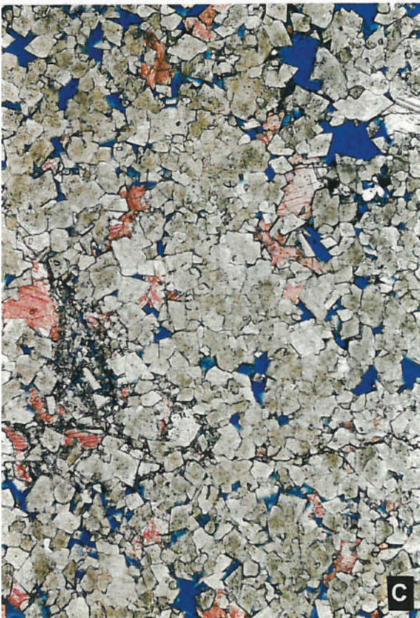
Very fine to fine crystalline dolomite, abundant planar-E interlocked with mosaics planar-S primarily intercrystalline porosity with scattered calcite void filling. 7107 ft.; X25
