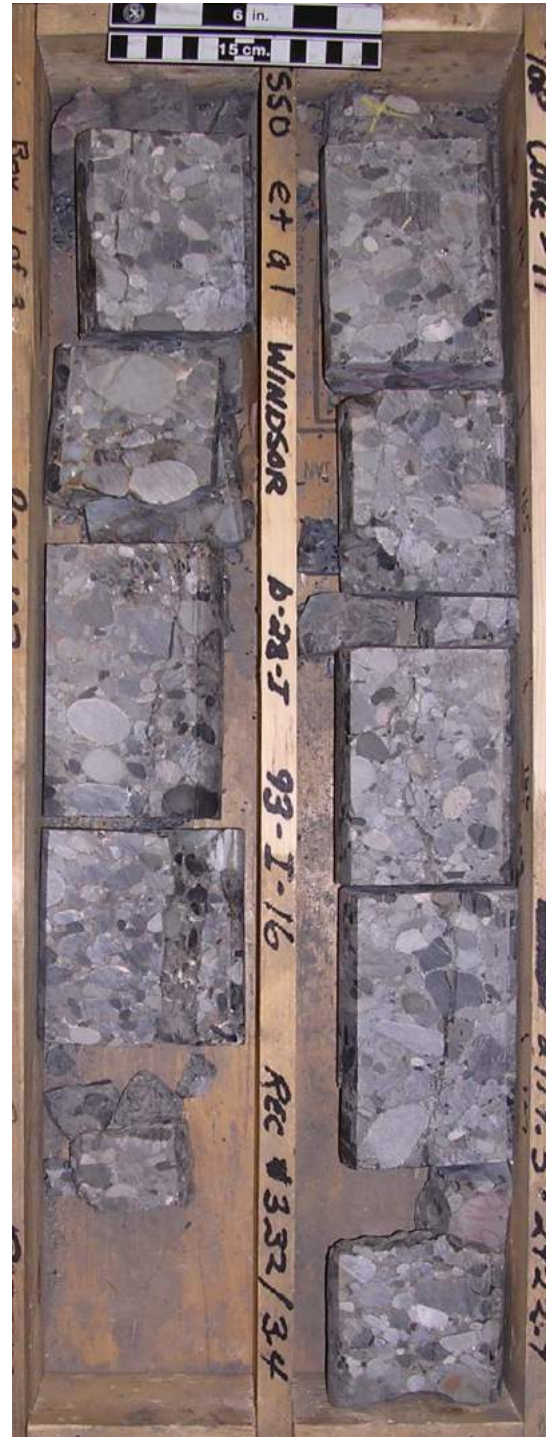
Typical poorly-sorted, brittle Cadomin conglomerate exhibiting extensive subvertical fracturing. b-28-1/93-1-16; 2919.5-2920.7 m.
