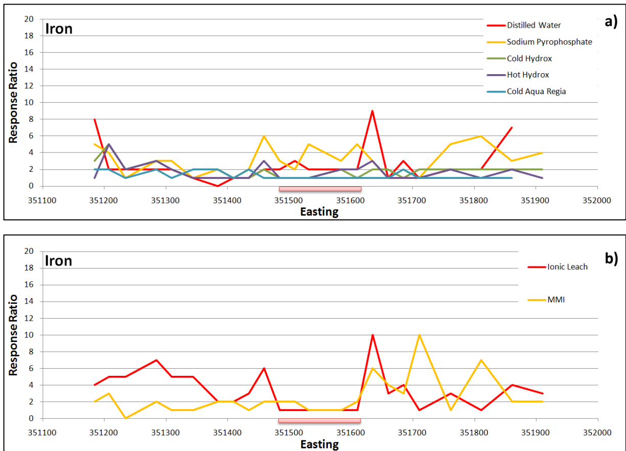
FIGURE 42. TRANSECT 1 - SELECTIVE AND PARTIAL EXTRACTION RESULTS FOR IRON. A. GENERIC EXTRACTION METHODS. B. LABORATORY SPECIFIC EXTRACTION METHODS.
