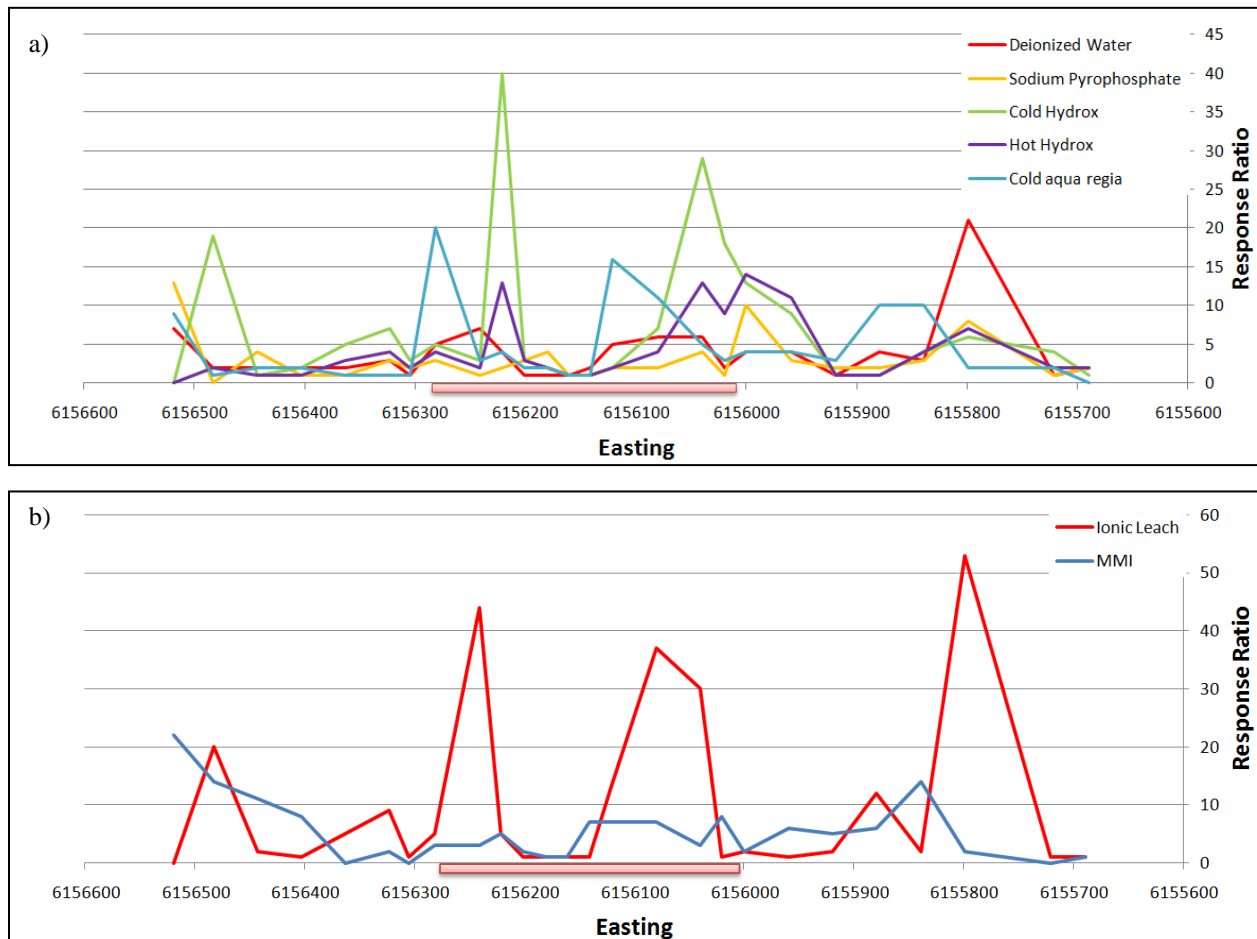
FIGURE 57. TRANSECT 2 - RATIO OF WEAK EXTRACTION CALCIUM TO AQUA REGIA CALCIUM. A. GENERIC EXTRACTION METHODS. B. LABORATORY SPECIFIC EXTRACTION METHODS.
