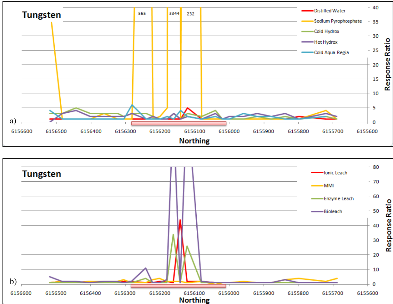
FIGURE 51. TRANSECT 2 - SELECTIVE AND PARTIAL EXTRACTION RESULTS FOR TUNGSTEN. A. GENERIC EXTRACTION METHODS. B. LABORATORY SPECIFIC EXTRACTION METHODS. NUMBERS AT THE TOP OF FIGURE 51A INDICATE THE MAXIMUM RESPONSE RATIOS.
