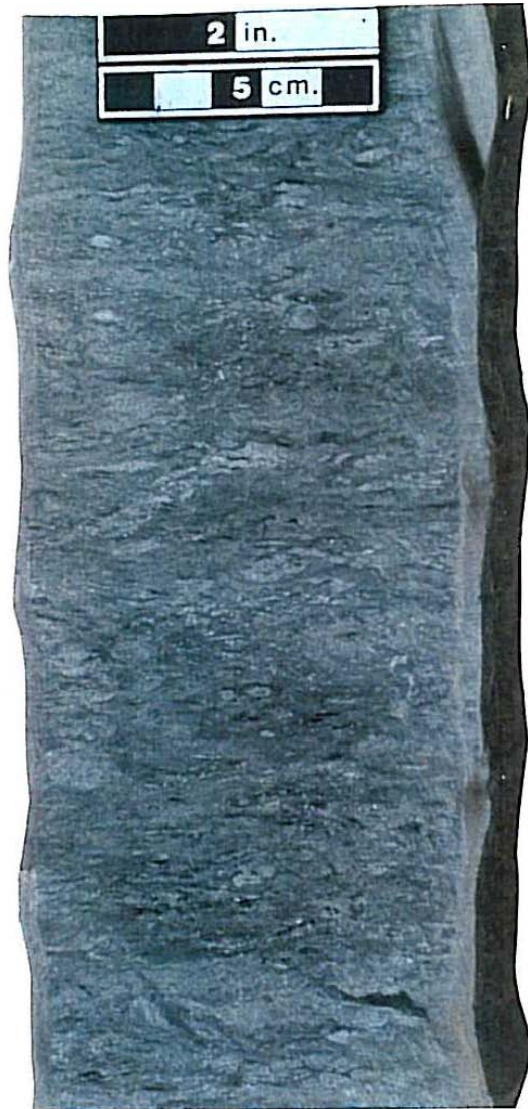
Figure B2. Pervasively burrowed Bluesky distal shoreface sandstone/mudstone. Mobil Sahtaneh a-8-B/94-I-13, 616.5 m.
