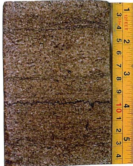
Figure R2. Massive, well-sorted and compacted coarse crinoidal limestone (packstone/grainstone), planar-bedded. Wincan et al Kimea d-57-D/94-P-10, 439 m ( \emptyset 7.7%, K 2.3 mD).
