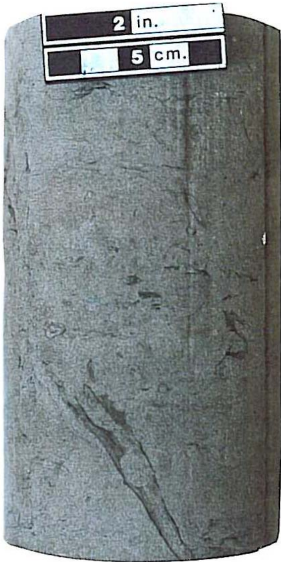
Figure B1. Bluesky shoreface sandstone with prominent Cylindrichnus ( Rosselia ?) burrow. Cdn Reserve Quintana Kotcho b-68-H/94-I-14, 1964 ft. (Core analysis \emptyset 20.4%, K 32 mD).
