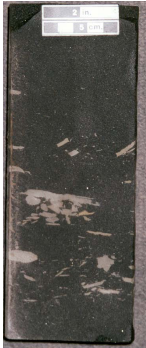
Figure M4. Sandstone, fine-grained, with pervasive pyrobitumen. Thin, flat mudstone rip-up clasts are not stained. ARCO Maxhamish b-21-K/94-O-14, 5375 ft.
