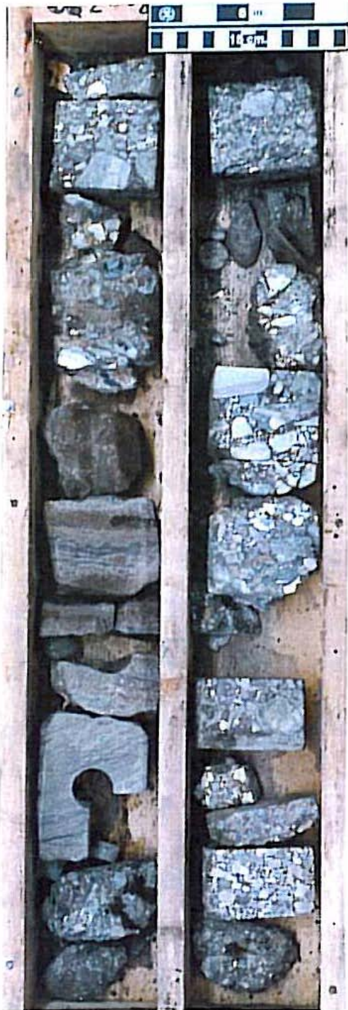
Figure G3. Interbedded poorly-sorted Gething conglomerate with sandstone matrix, and argillaceous sandstone. Mobil North Petitot d-33-E/94-P-13, 298-299.2 m (Core analysis Ø 14-22%, K 44-396 mD).
