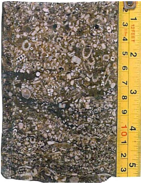
Figure R1. Massive, very coarse-grained crinoidal limestone (grainstone/packstone), oil-stained. Mobil North Petitot d-97-C/94-P-13, 362.5 m ( \emptyset 11.6%, K 0.03 mD).
