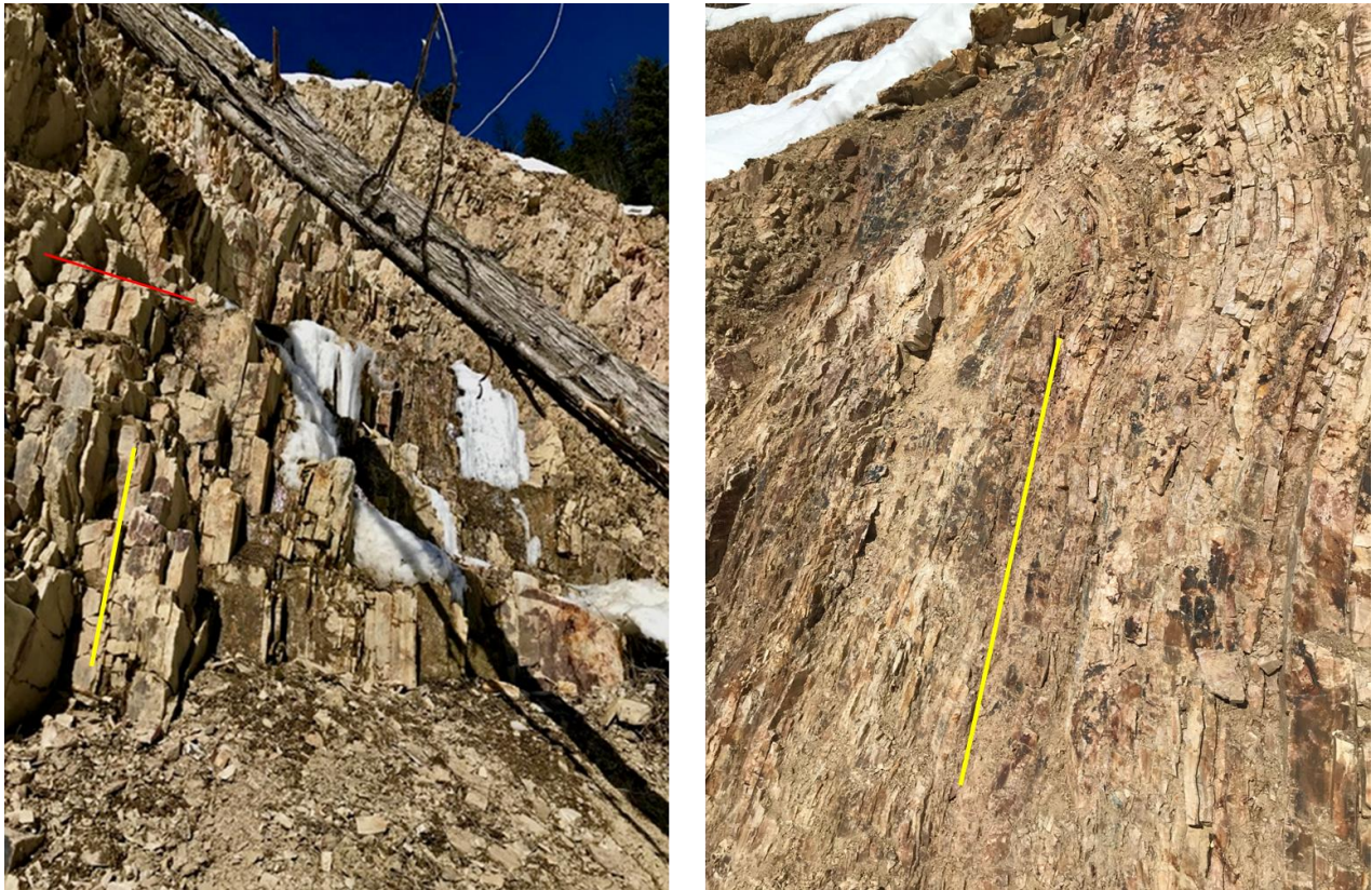
Figure 13 – Hamill quartzite exposure along the Orebin Creek Fault, Fault gouge zone shown on the right (Strike 180° (yellow), Dip 86° West; Joint set Strike 118° (red), Dip 69-73°)
