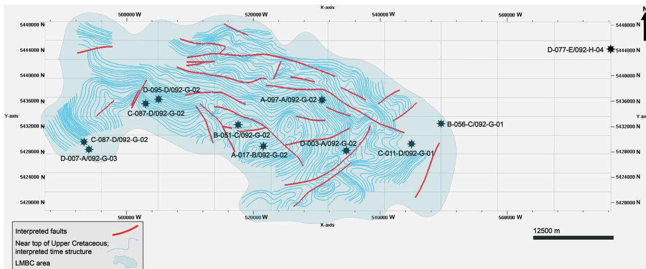
**Figure 9.** Seismic time structure map of the Upper Cretaceous and the interpreted faults in the Lower Mainland, British Columbia (LMBC). Also shown are the locations of wells (unique well identifiers; BC Oil and Gas Commission, 2022) from which data were obtained. The digitized version of the interpretation of the Upper Cretaceous horizon and faults in the LMBC area was prepared using Schlumberger Limited’s Petrel software.
