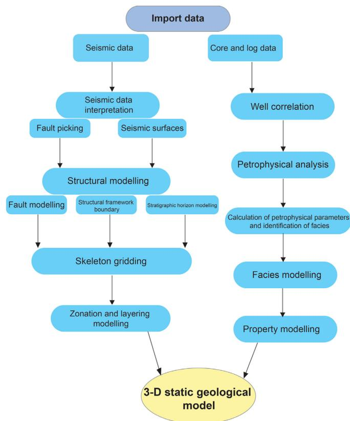
**Figure 10.** Flow chart of the three-dimensional (3-D) static geological modelling process.
