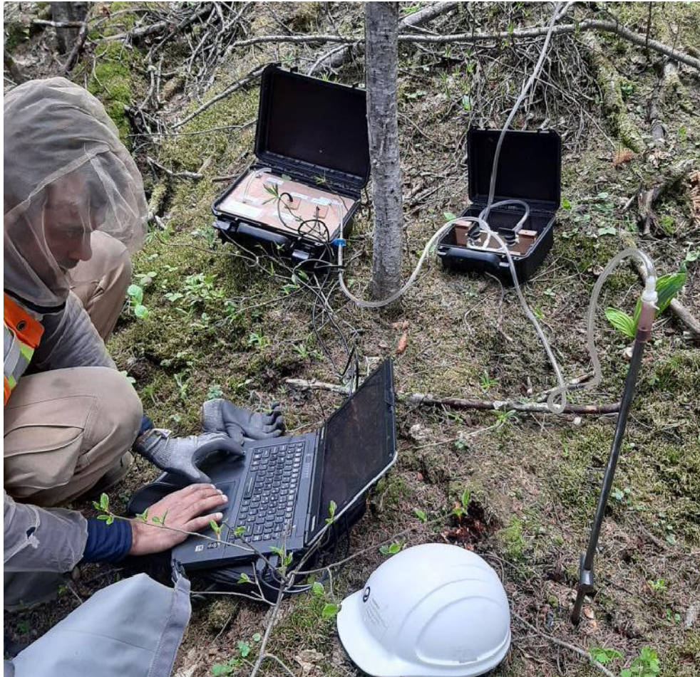
Figure 4. The modified soil gas collection-analysis system showing the sensor and shut-off valve unit, soil probe and lap top computer during the Mount Milligan survey.
