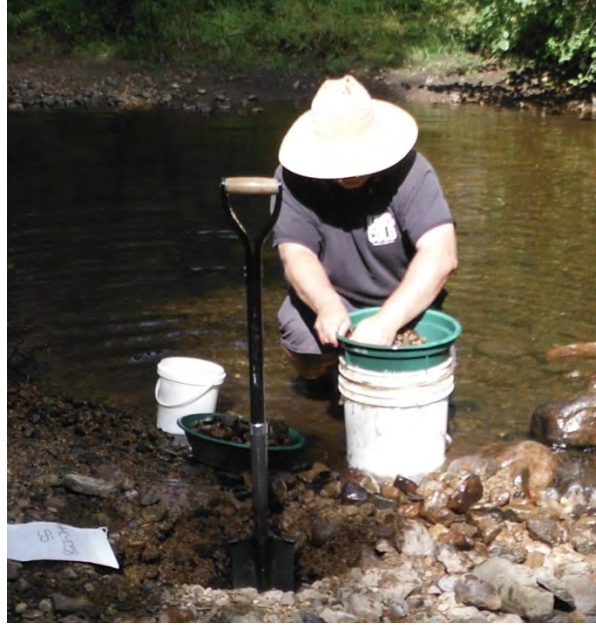
Figure 3. A representative bulk stream-sediment pit located on a mid-channel bar and sieving of sample material to capture the minus 10 mesh material in a 20 litre plastic bucket.
