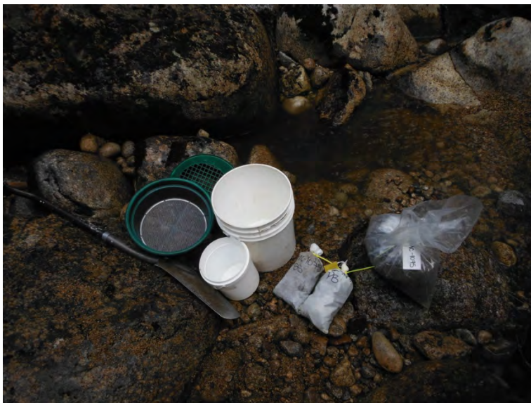
Figure 2. Sampling equipment used to collect stream-sediment samples, including bulk stream sediment collected into polyethylene sample bag plus silt-sediment and pebbles samples in synthetic cloth bags.
