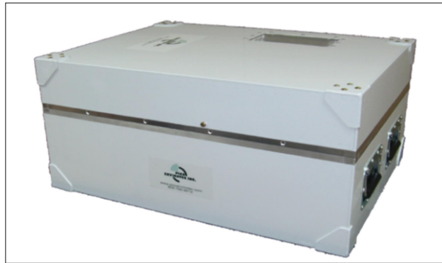
Figure 24: AGRS-5 gamma spectrometer system with five detectors; a total of 21 litres NaI(Tl) synthetic crystals with 4 down and 1 up.
