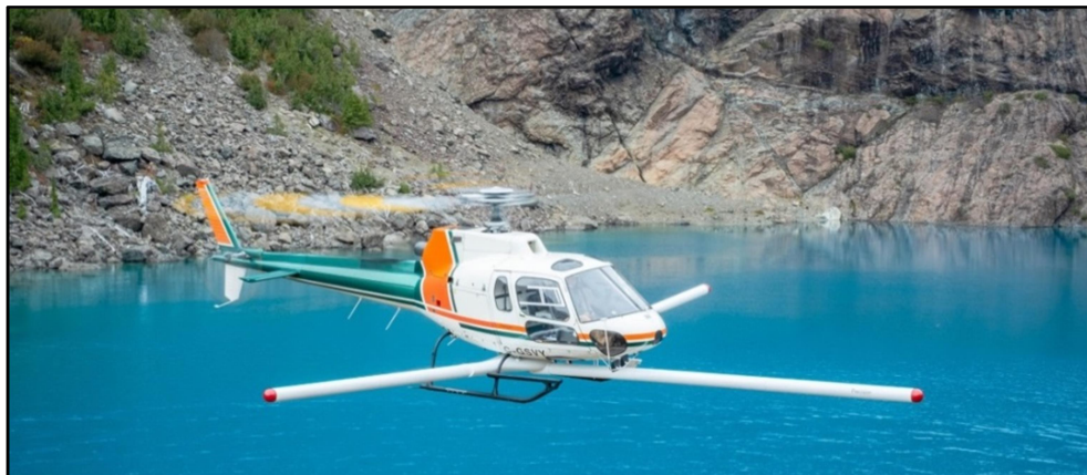
Figure 22: View of triple magnetic boom system used on Vancouver Island North survey. One magnetometer installed at the end of each boom to provide total magnetic intensity, crossline magnetic gradient, and inline magnetic gradient measurements.
