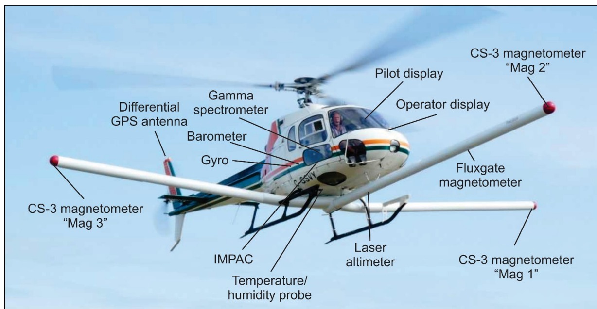
Figure 19: Airbus AS350 "AStar" helicopter equipped with three magnetic sensors for magnetic data acquisition and internal 21 litres of gamma crystals for radiometric data acquisition.
