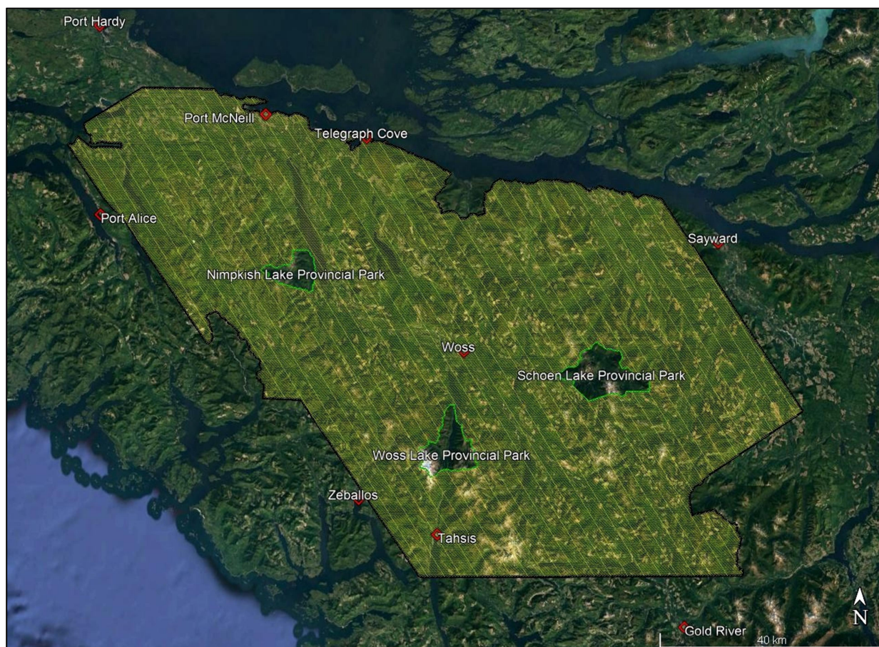
Figure 3: Plan View – Vancouver Island North survey block with actual flight lines in yellow, survey block boundary in black, and provincial parks in green.
