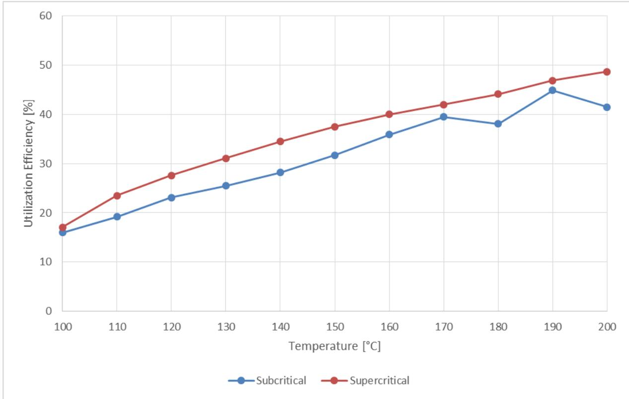
Figure 16 Optimal utilization efficiencies of sub- and supercritical binary cycle geothermal power plants. Graph based on data by Augustine (2014).
