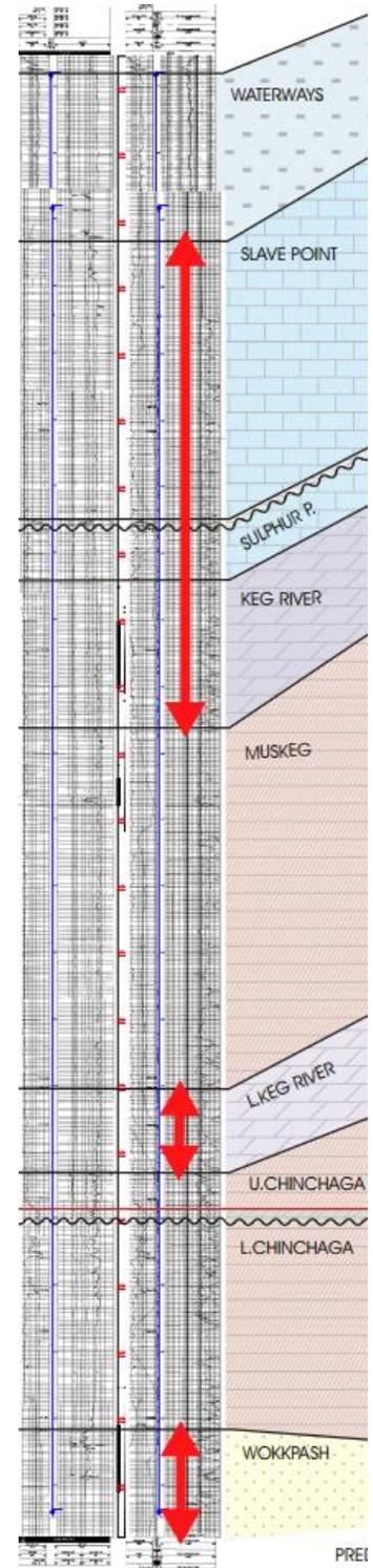
Figure 12 Example of reservoir thickness assessment for well 00/A-011-D/094-J-07/4. Red arrows indicate strata considered permeable for thickness estimate.
