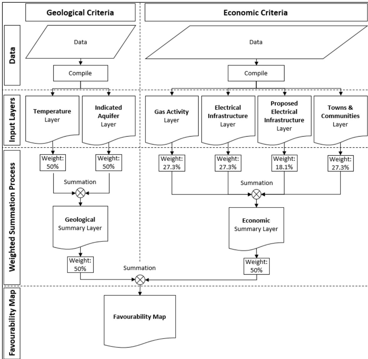
Figure 2 Overview Flowchart of the process to compute the favourability map, employing an adaptation of a two-level Weighted Linear Combination
