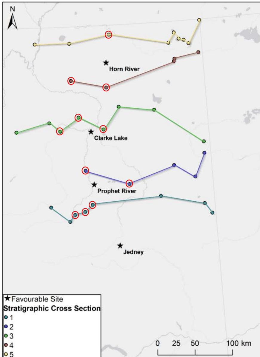
Figure 11 Location of stratigraphic cross sections used for reservoir thickness estimation. Well locations highlighted in red are used for reservoir thickness estimation. Cross sections were compiled by Ibrahimbas & Walsh (2005).
