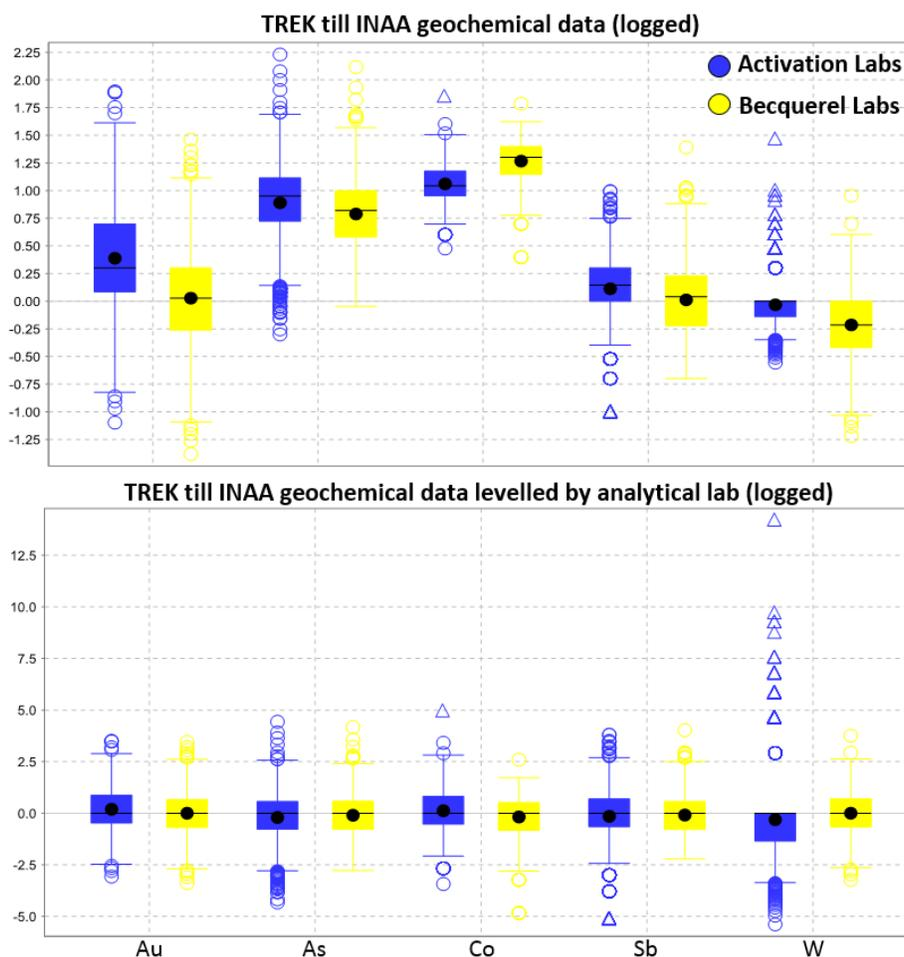
**Figure 8.** Box plots comparing analytical results from INAA for each lab before (top) and after (bottom) z-score levelling. The levelling procedure converts each value to a group-based z-score. After levelling, all groups have a mean of 0 (black dot on box plots) and a standard deviation of 1. The z-score levelling method does not change the shape of the distribution and genuine outliers are preserved.
