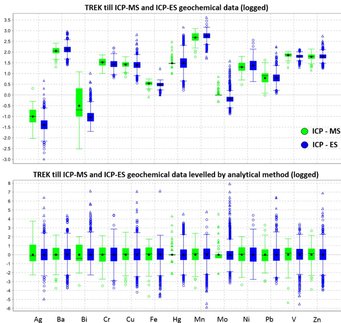
**Figure 7.** Box plots comparing analytical results from ICP-MS and ICP-ES before (top) and after (bottom) z-score levelling. The levelling procedure converts each value to a group-based z-score. After levelling, all groups have a mean of 0 (black dot on box plots) and a standard deviation of 1. The z-score levelling method does not change the shape of the distribution and genuine outliers are preserved.
