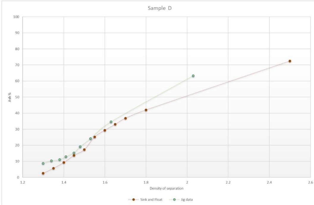
Figure 13b. Density of separation (S.G. and ARD) vs. ash in density fractions for sample D.
