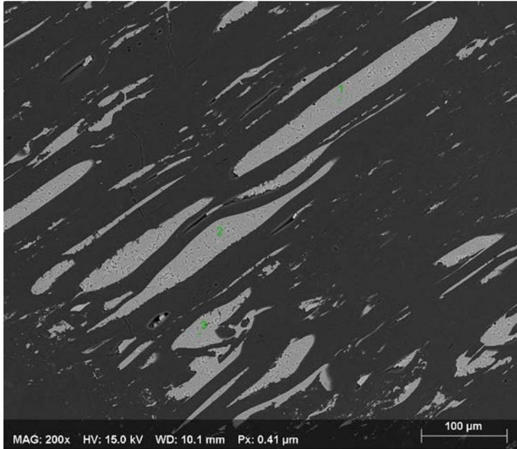
Figure 4. Fusinite pores filled with possible Kaolinite ( $\text{Al}_2(\text{Si}_2\text{O}_5)(\text{OH})_4$ ). Numbers represent EDX analysis locations where elements Si, O, and Al were detected.
