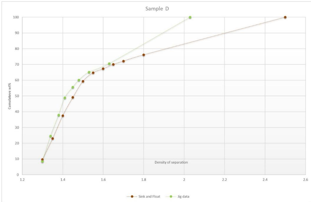
Figure 13c. Density of separation vs. cumulative yield of clean coal for sink and float and jig procedures.
