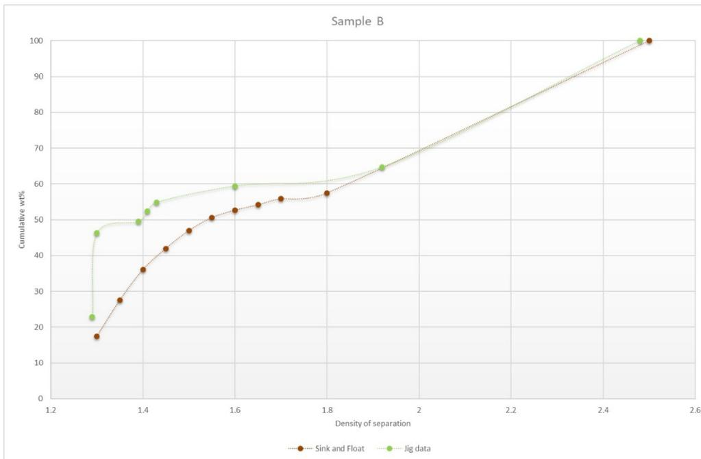
Figure 11c. Density of separation vs. cumulative yield of clean coal for sink and float and jig procedures.
