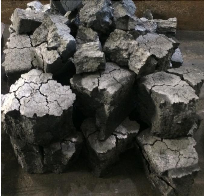
Figure 8 – Sole-heated oven coke from Coal Sample C cleaned using the Float-sink method.
