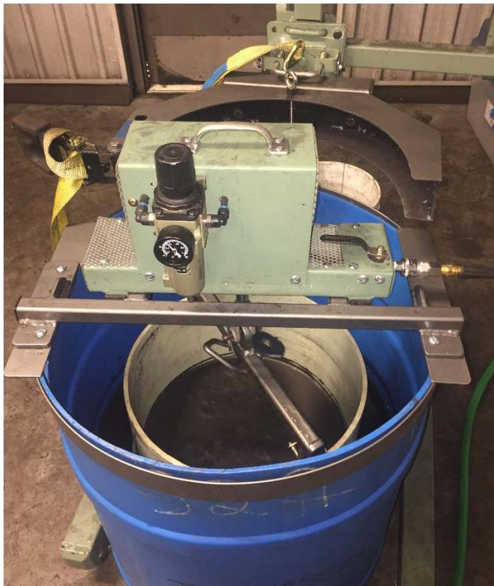
Figure 4. The Roben Jig equipment used in this study.
