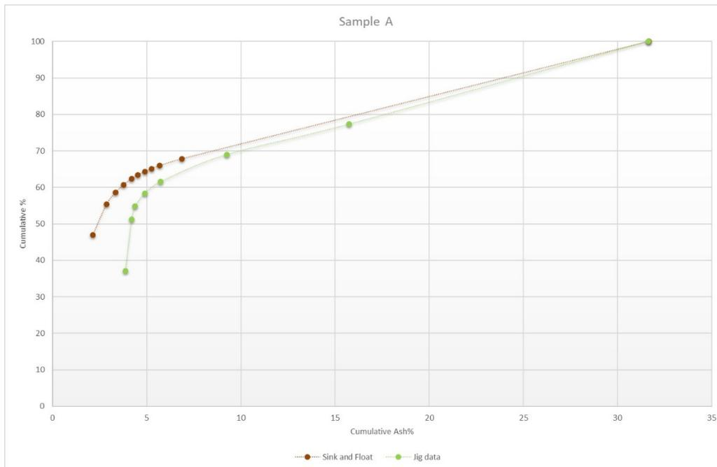
Figure 10a. Clean coal curve for sample A.
