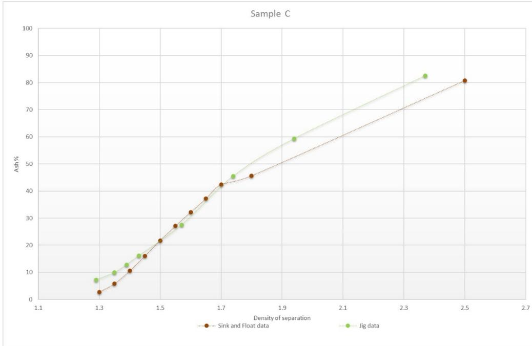
Figure 12b. Density of separation (S.G. and ARD) vs. ash in density fractions for sample C.
