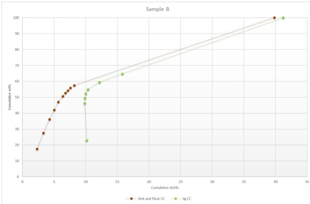
Figure 11a. Clean coal curve for sample B.
