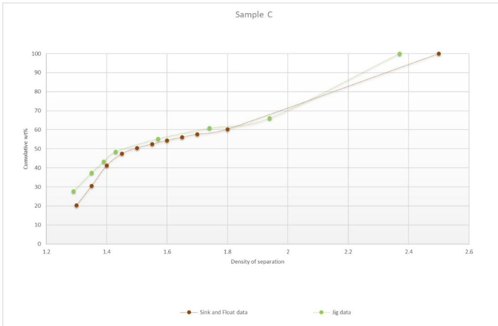
Figure 12c. Density of separation vs. cumulative yield of clean coal for sink and float and jig procedures.
