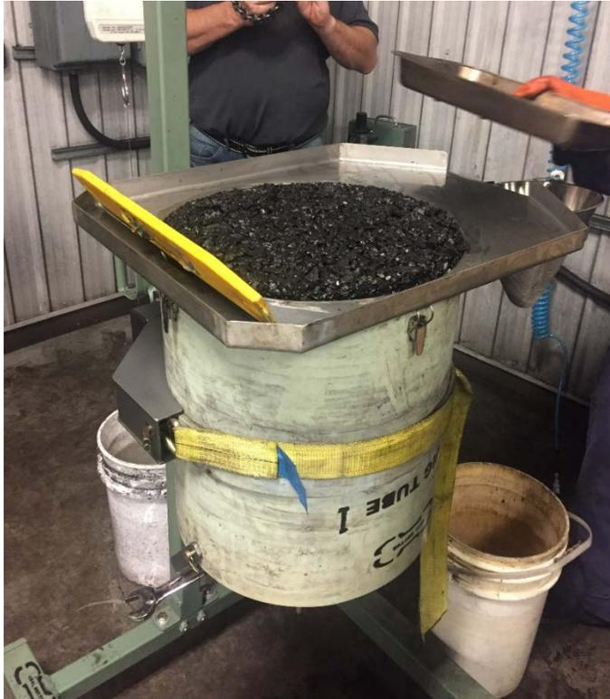
Figure 5. Inverted Roben Jig with coal slice ready to be removed.
