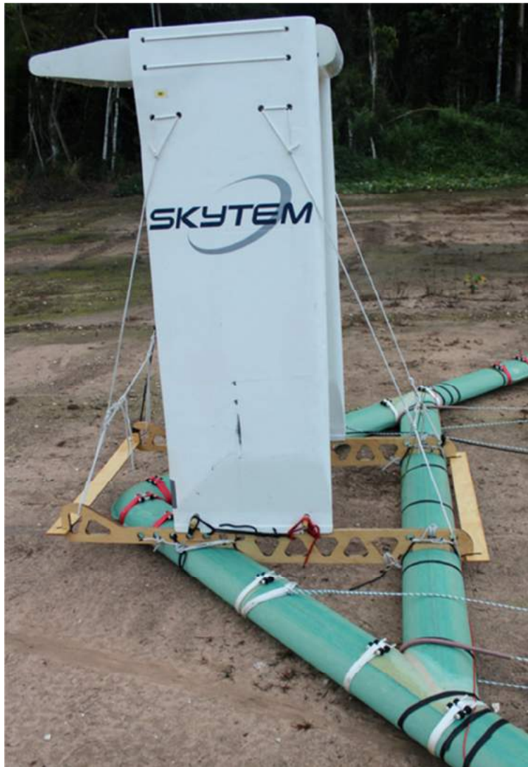
Figure 3 Rudder containing the Z coil located in the top part of the tower.
