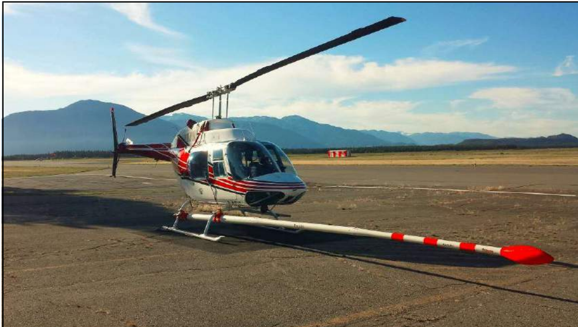
Figure 19: Bell 206B JetRanger helicopter C-GTVL at Terrace airport (CYXT) equipped with mag stinger for magnetic data acquisition.
