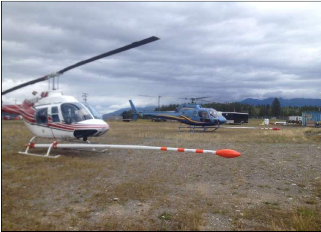
Figure 22: View of mag stinger installed on Bell 206B C-GTVL, used on Search 2015 survey.
