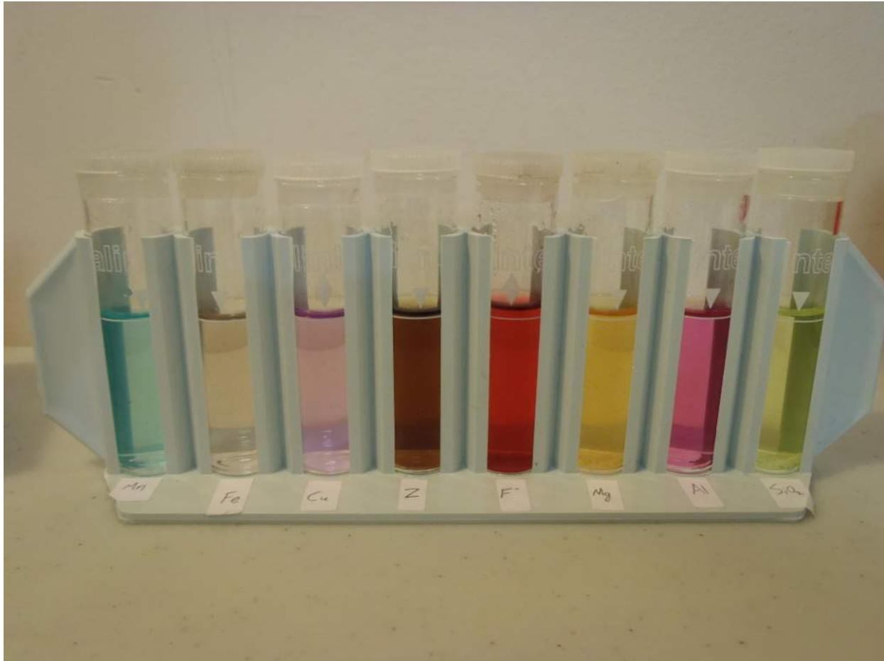
Figure 5. Close-up of rack showing a collection of tubes with reagents ready for photometer testing.
