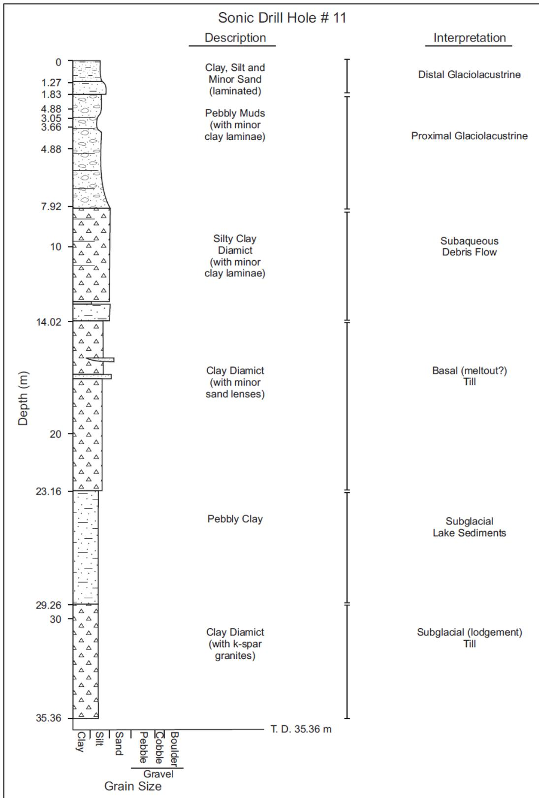
Figure 24. Stratigraphic log and interpretation of main units at sonic drill hole 11
