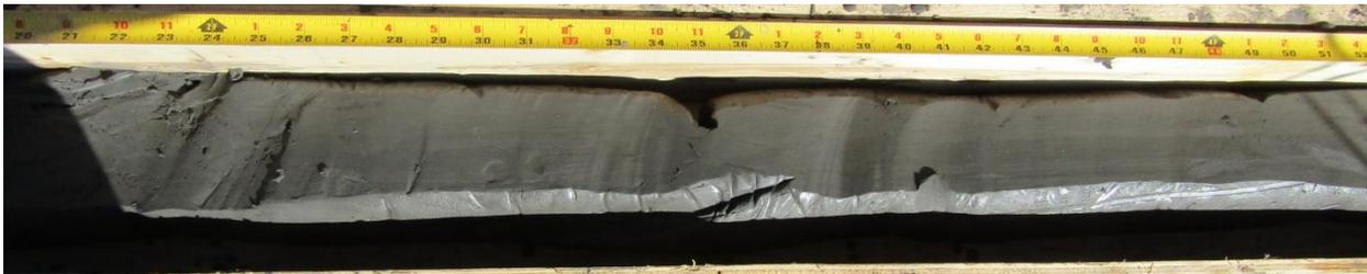
Figure 12. Laminated silts and clays in sonic hole 7 at a depth of about 31.7 m (103-105 ft)
