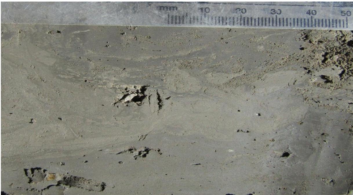
Figure 5. Close-up view of thin silt laminae (light grey) in thicker clay beds (dark grey) in sonic hole 3; deformation mainly from drilling; note small pebble in photo centre (scale in mm)
