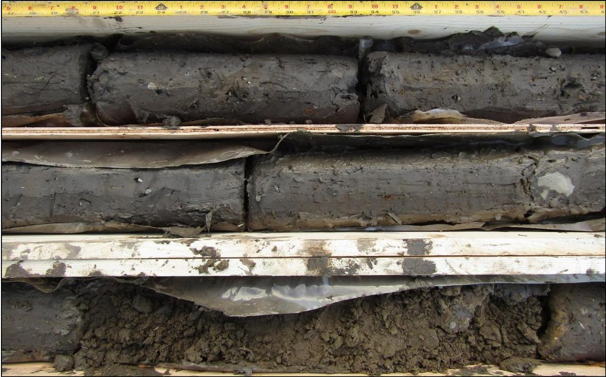
Figure 27. Fine to coarse sand bed at about 16.5 m depth (lower box, 53-55 ft) in sharp contact with silty-clay diamict at about 14-16 m depth (upper boxes) in sonic hole 12
