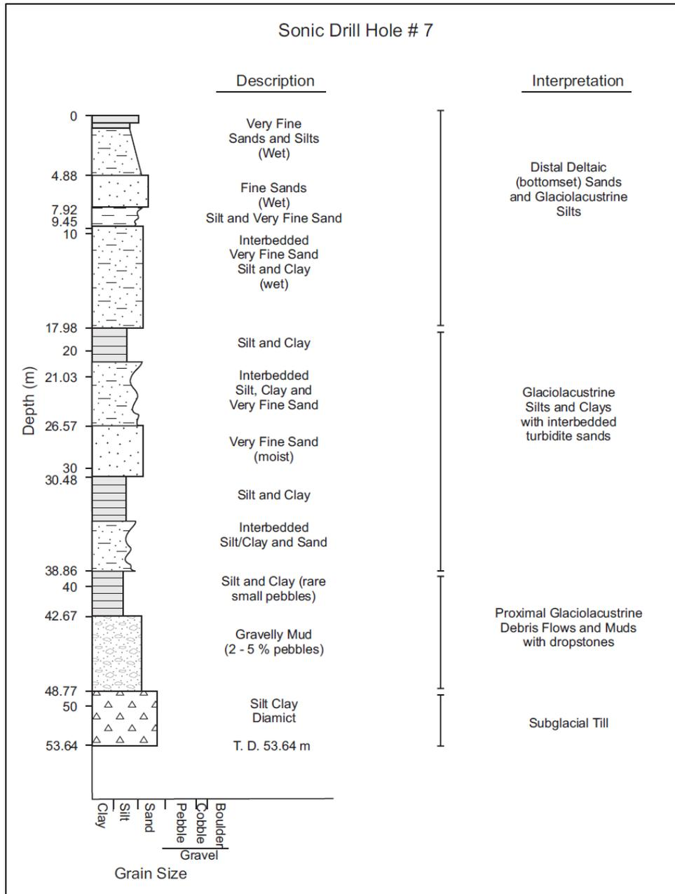
Figure 10. Stratigraphic log and interpretation of main units at sonic drill hole 7
