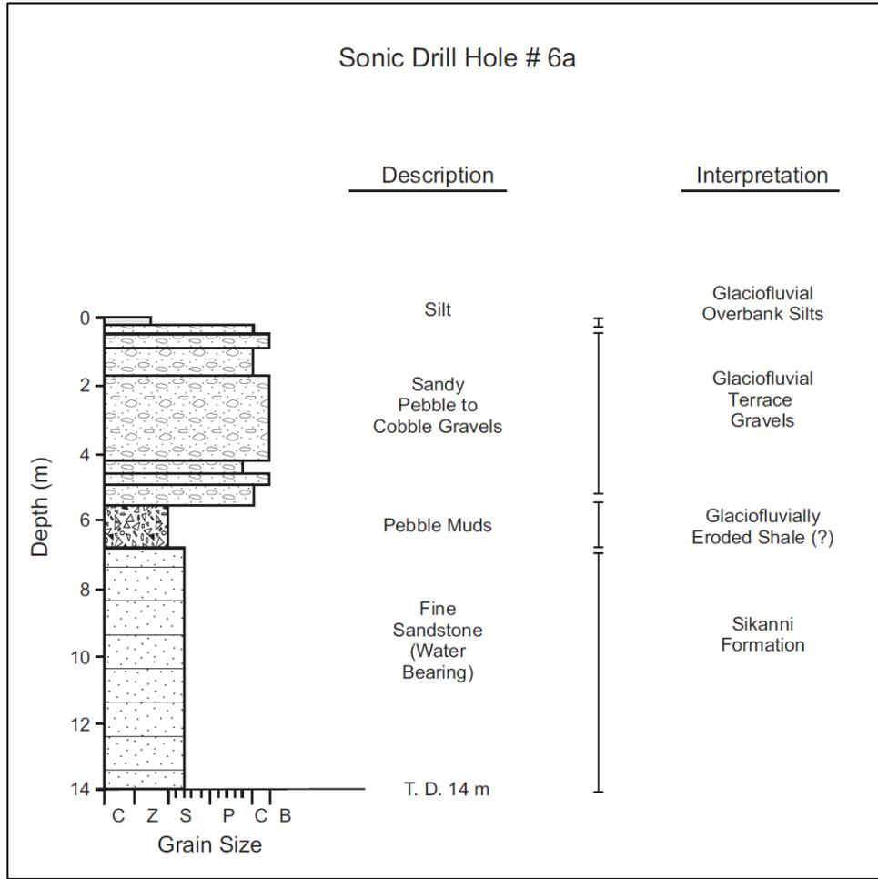
Figure 7. Stratigraphic log and interpretation of main units at sonic drill hole 6a
