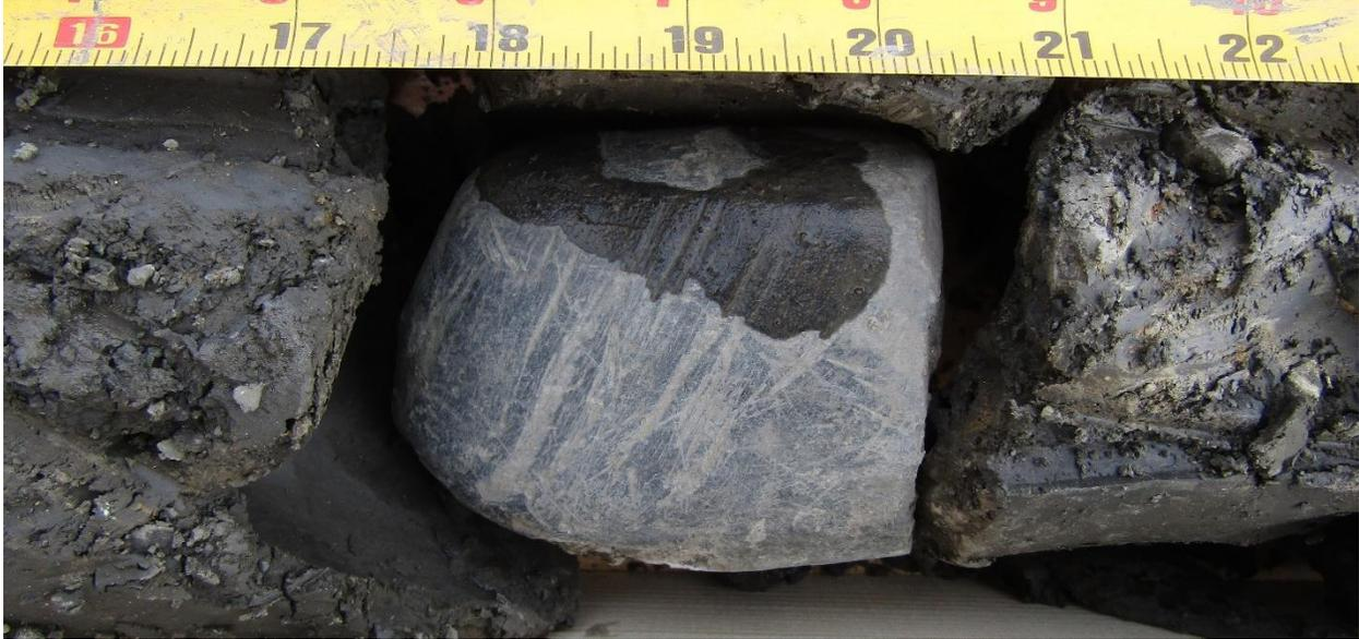
Figure 22. Striated and faceted clast in dense, massive diamict interpreted as basal till at a depth of about 51.8 m (170 ft) in sonic drill hole 10x; scale in inches
