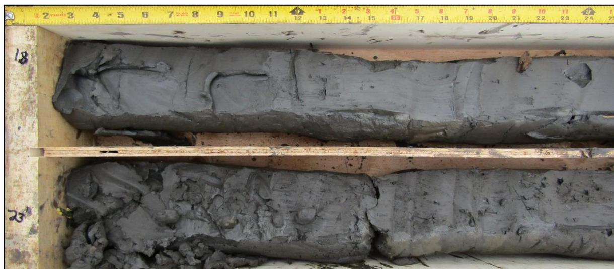
Figure 30. Rhythmically bedded silts and clays in sonic drill hole 13 at about 5.5-7.5 m depths (intervals shown: top box 18-20 ft, bottom box, 23-25 ft), interpreted to be varved glaciolacustrine sediments
