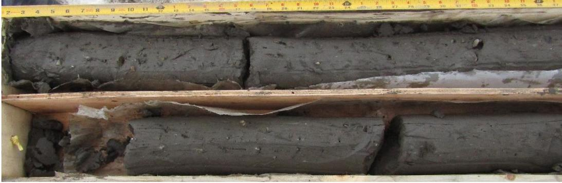
Figure 25. Massive, matrix-supported, very dense, clay rich diamict at a depth of about 33 m in sonic hole 11 (depth interval shown: 104-107 ft, top box, and 108-111 ft, bottom box) interpreted to be subglacial lodgement till deposited at the base of the Laurentide Ice Sheet
