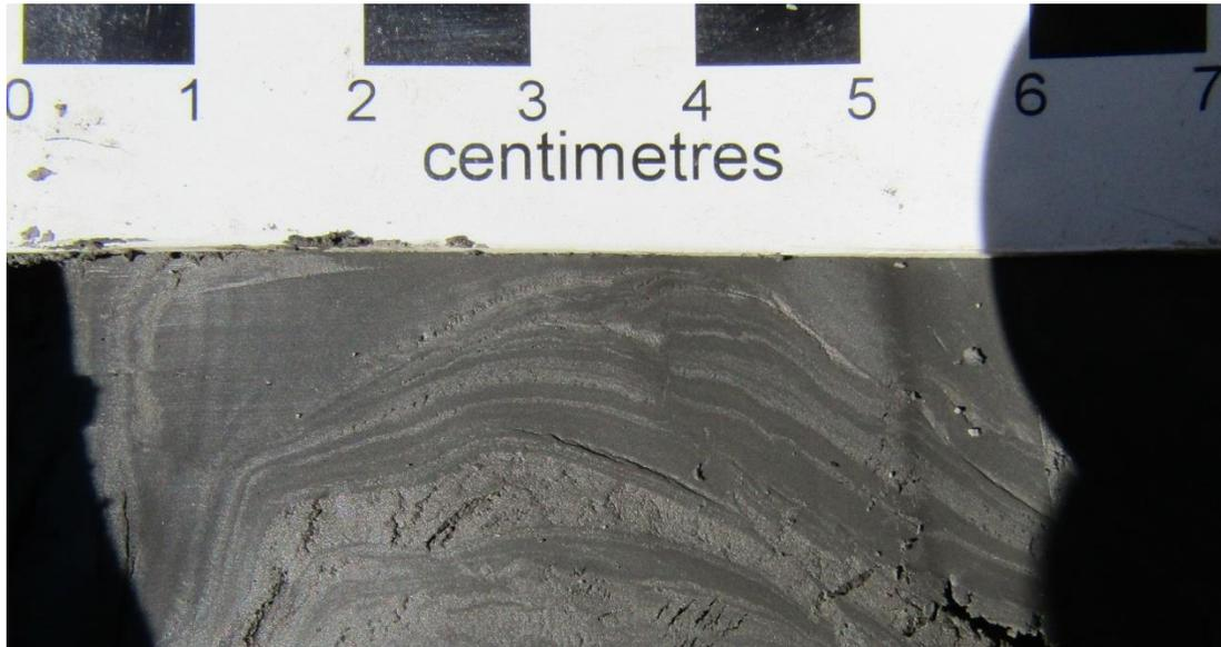
Figure 13. Close-up of well laminated silts and clays (dark grey) and fine sands (light grey) in sonic hole 7; deformation, especially on the lateral margins of the core, is assumed to be from drilling disturbance
