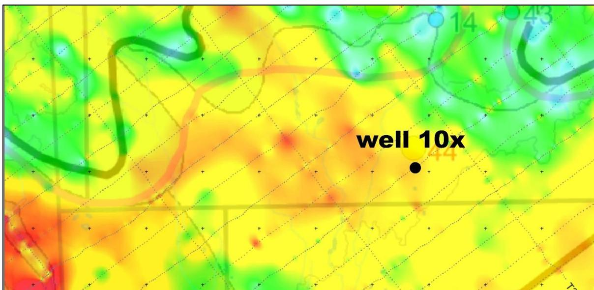
Figure 18. Location of well 10x on the 15-20 m resistivity depth slice
