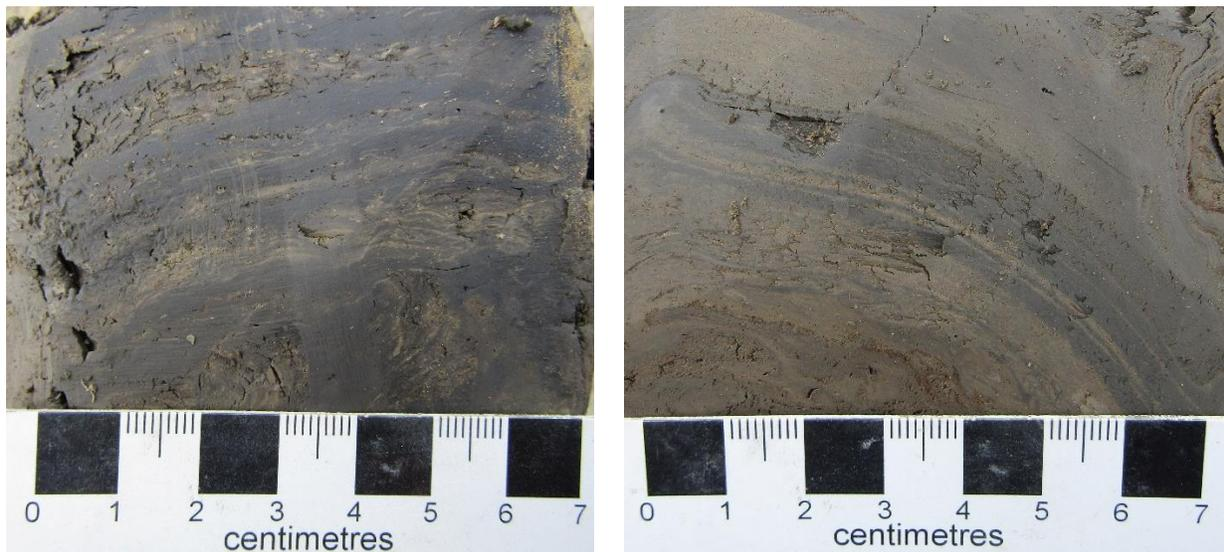
Figure 15. Close-up views of well laminated silts (light brown) and clays (dark grey) in sonic hole 10b at about 1.5 m (5 ft) depth (Left photo) and about 24.7 m (81 ft) depth (Right photo); deformation induced by drilling
