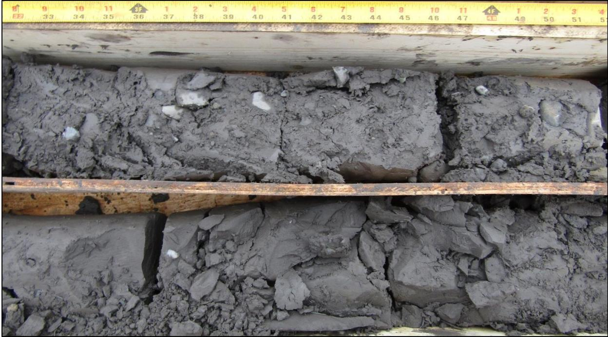
Figure 34. Massive, gravelly silts and fine sands at about 45.7 m (top box, 149-151 ft) interbedded with pebbly fine sands at about 47 m (bottom, 154-156 ft) in sonic hole 13, interpreted to be glacial debris flow deposits
