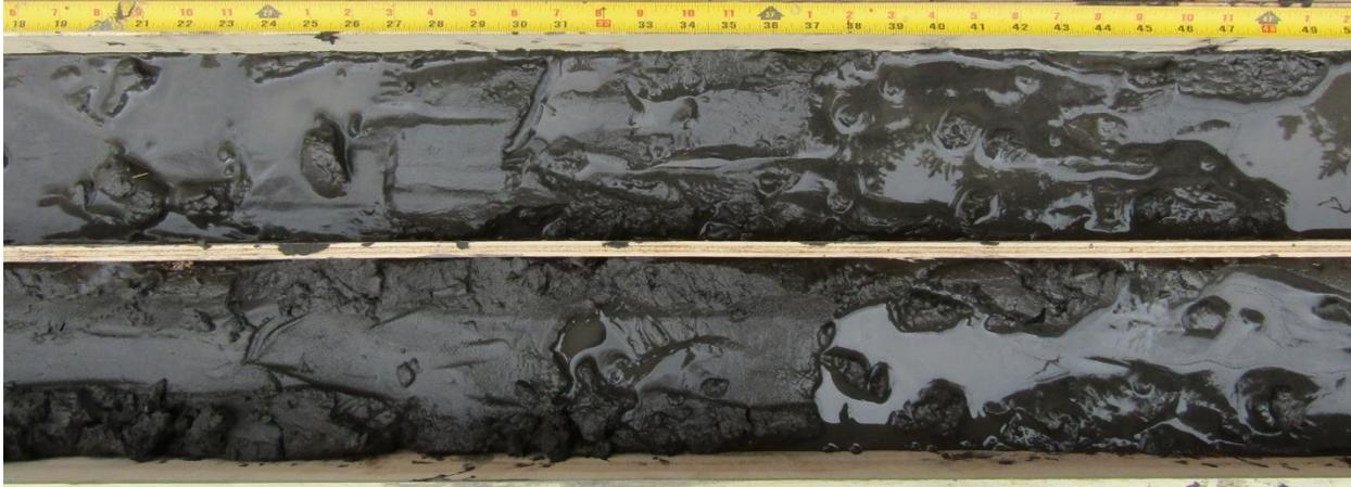
Figure 11. Liquefied fine to very fine sands in sonic hole 7 at depths of about 13.5 m (top, 43-45 ft) and 14.3 m (bottom, 48-50 ft); scale in inches
