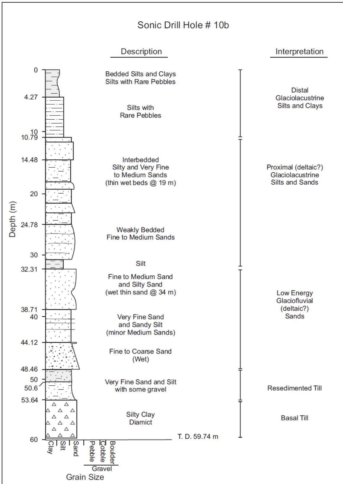
Figure 14. Stratigraphic log and interpretation of main units at sonic drill hole 10b
