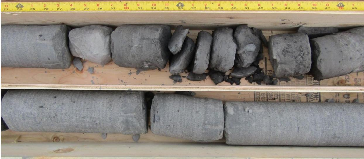
Figure 9. Fractured sandstone bedrock with minor shale partings in drill hole 6a at a depth of about 12 m (top 38-40 ft) and 13.5 m (bottom 43-45 ft)
