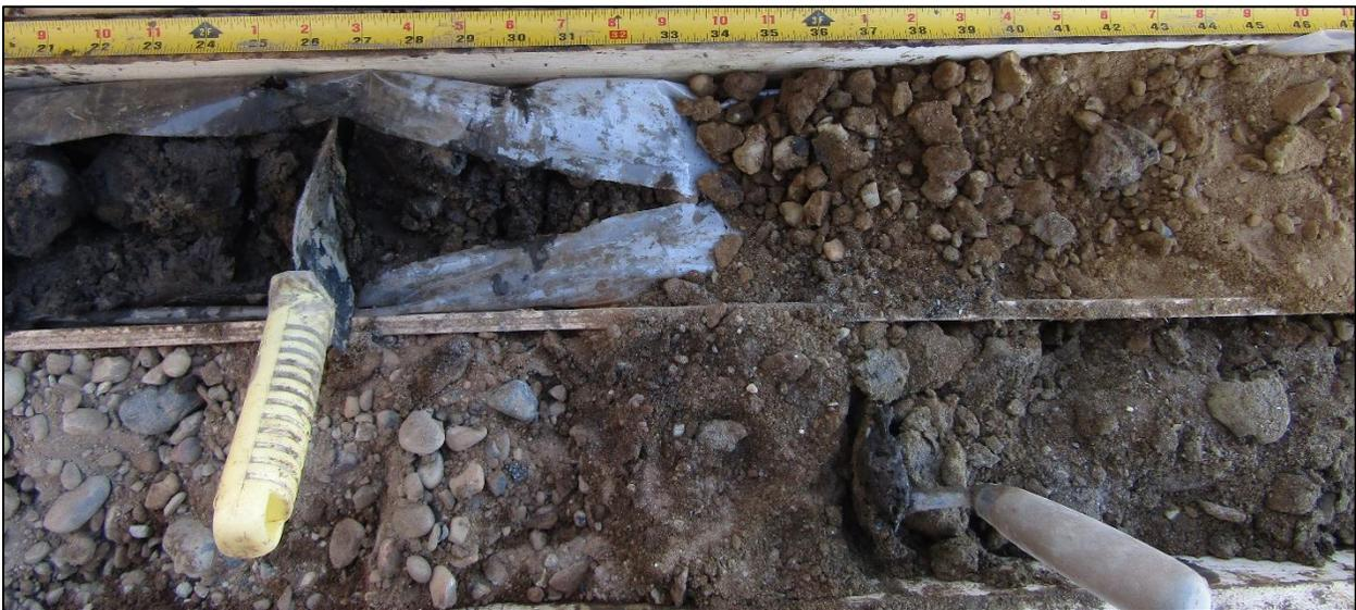
Figure 28. Dry sandy gravels at about 30 m depth (98-102.5 ft) in sonic hole 12; gravel top and bottom marked by trowel positions; scale in inches
