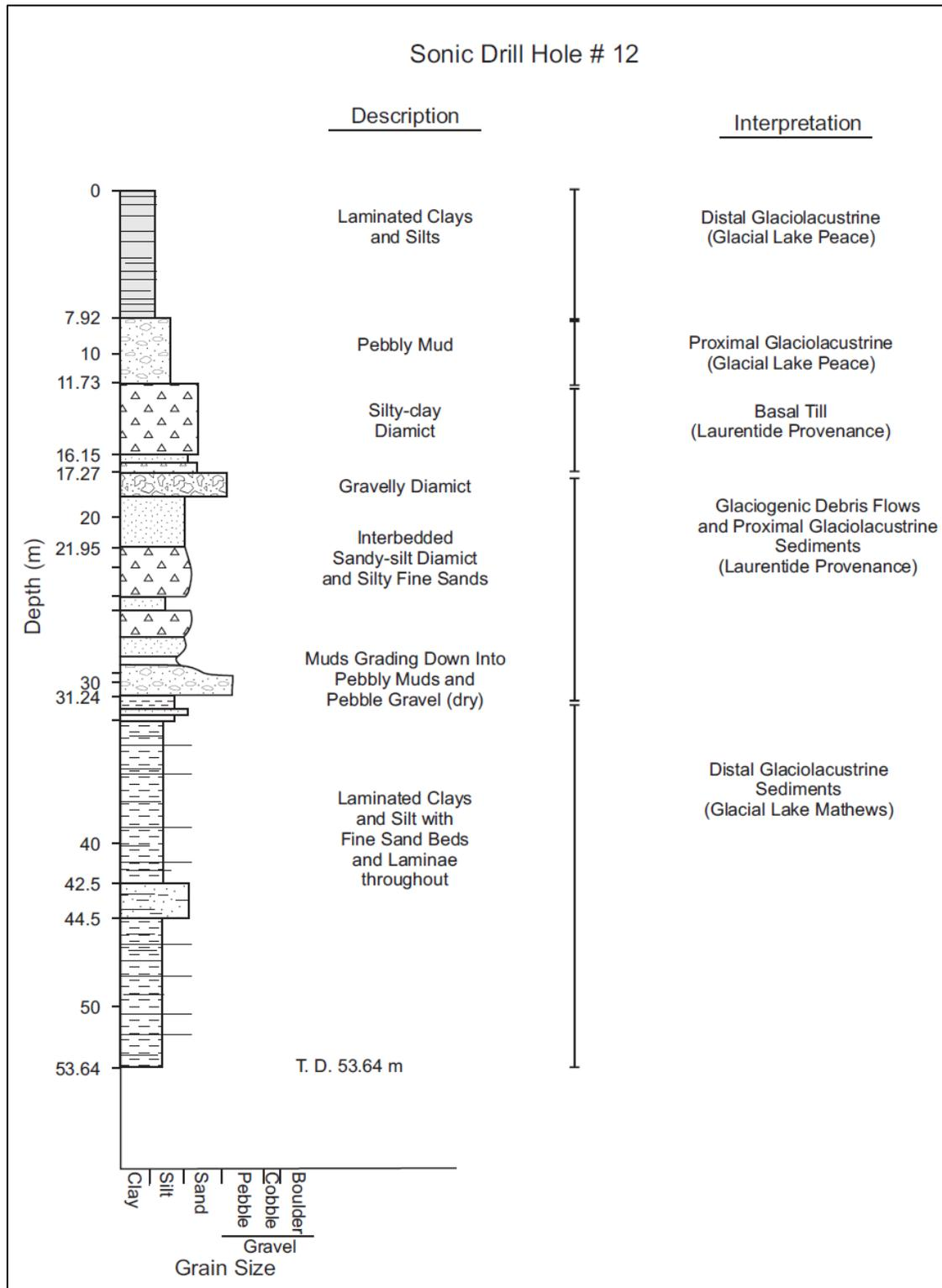
Figure 26. Stratigraphic log and interpretation of main units at sonic drill hole 12
