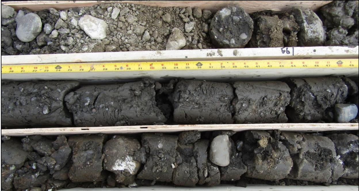
Figure 32. Thin glaciofluvial gravel at about 16.8 m depth (upper box, 55-55.5 ft) in sonic hole 13 overlying massive, dense diamict at about 18-20 m (lower boxes, 59-61 ft and 63-65 ft), interpreted to be Cordilleran basal till
