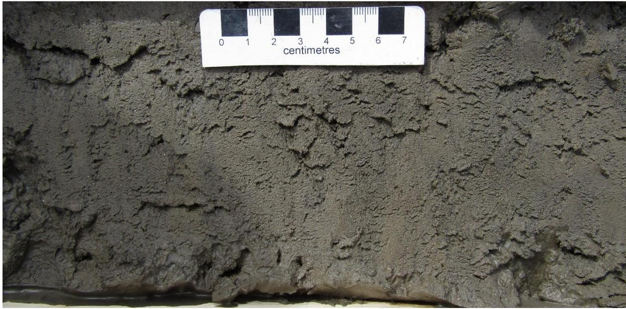
Figure 16. Close-up view of wet fine sand beds at about 19 m depth in sonic hole 10b
