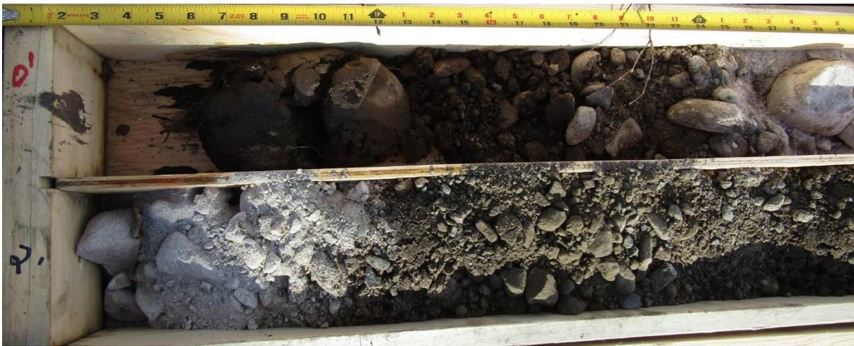
Figure 8. Thin overbank silt overlying quartzites and sandstone rich gravels in the upper metre at sonic hole 6a
