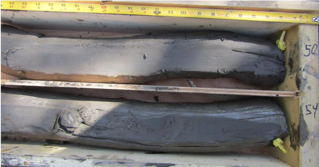
Figure 4. Soft clays and silts with minor pebble at a depth of about 15.5 m (48-50ft & 52-54ft) in sonic drill hole 3 interpreted to be glaciolacustrine sediments (scale in inches)
