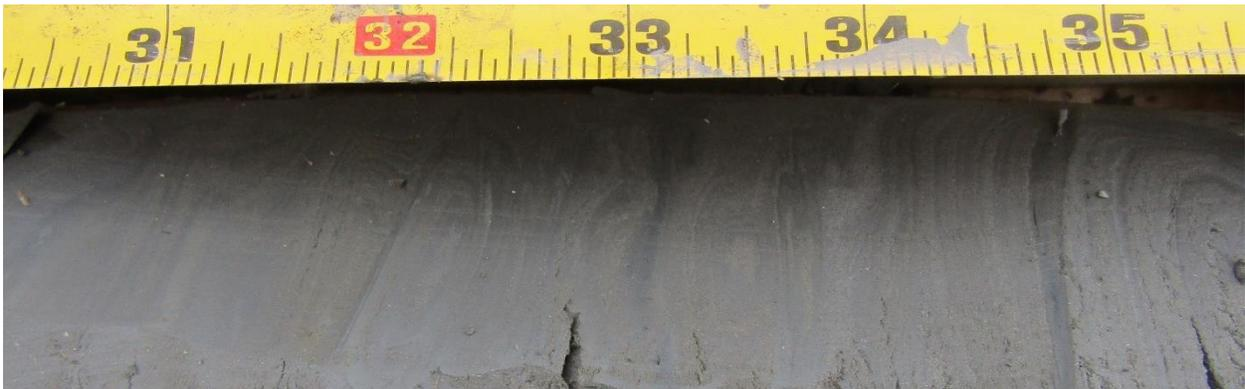
Figure 23. Well laminated, dense, silts and clays near the base of sonic hole 10x at a depth of about 60 m (197 ft); scale in inches
