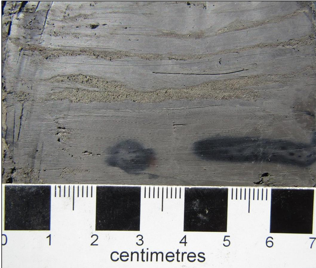
Figure 29. Dense, laminated, silts, clays and fine sands at a depth of about 50 m (134.5 ft) in sonic hole 12, interpreted to be sediments deposited in Glacial Lake Mathews; note black (organic?) zones at photo base
