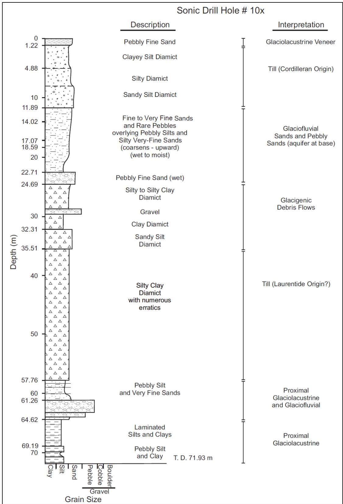
Figure 19. Stratigraphic log and interpretation of main units at sonic drill hole 10x
