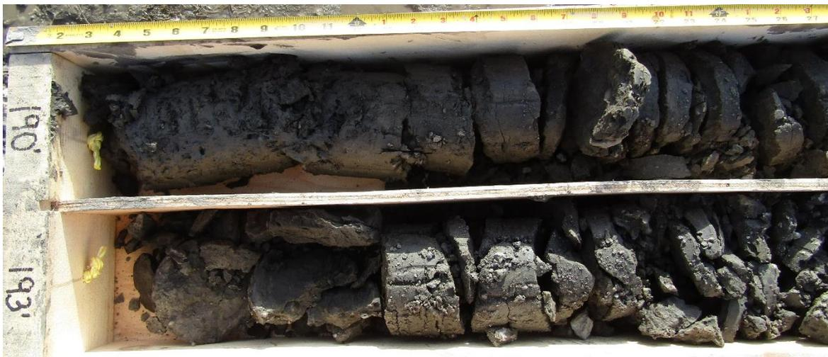
Figure 17. Massive, dense, matrix-supported diamict interpreted as basal till from a depth of about 58.5 m (190-194 ft) near the bottom of sonic drill hole 10b.
