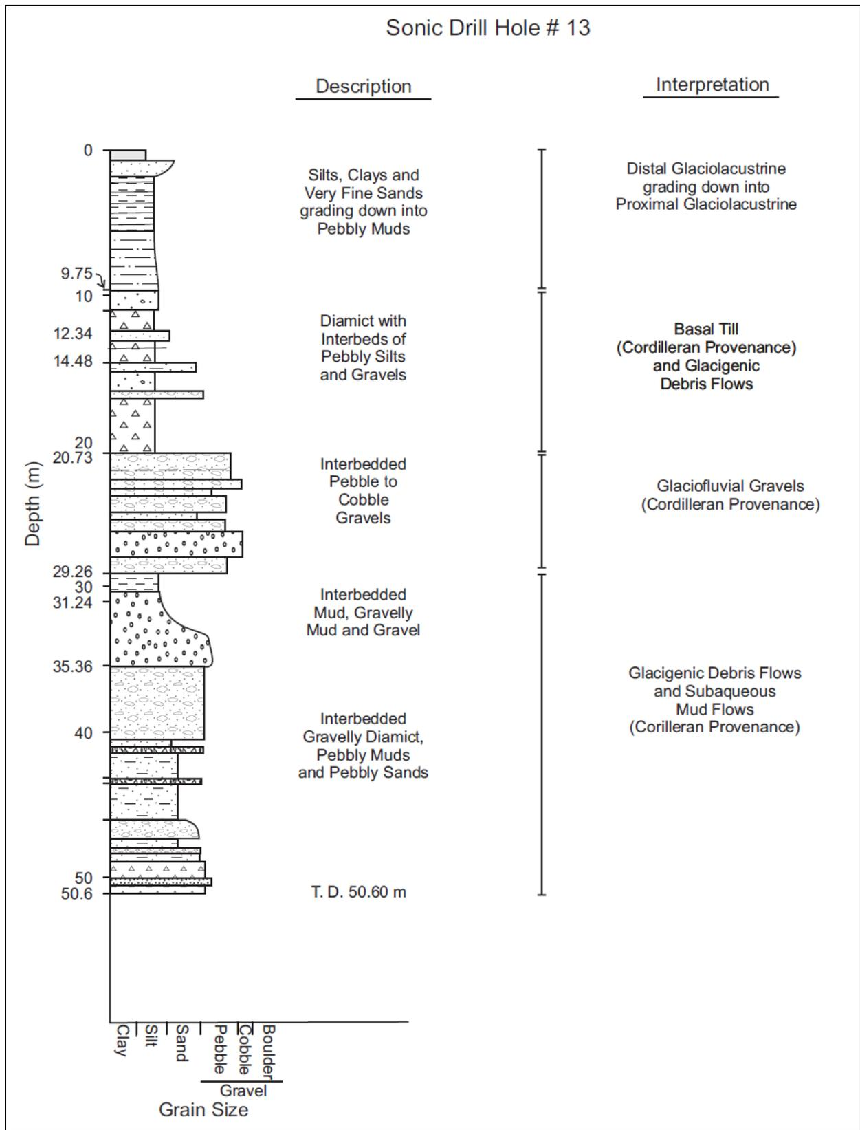
Figure 31. Stratigraphic log and interpretation of main units at sonic drill hole 13
