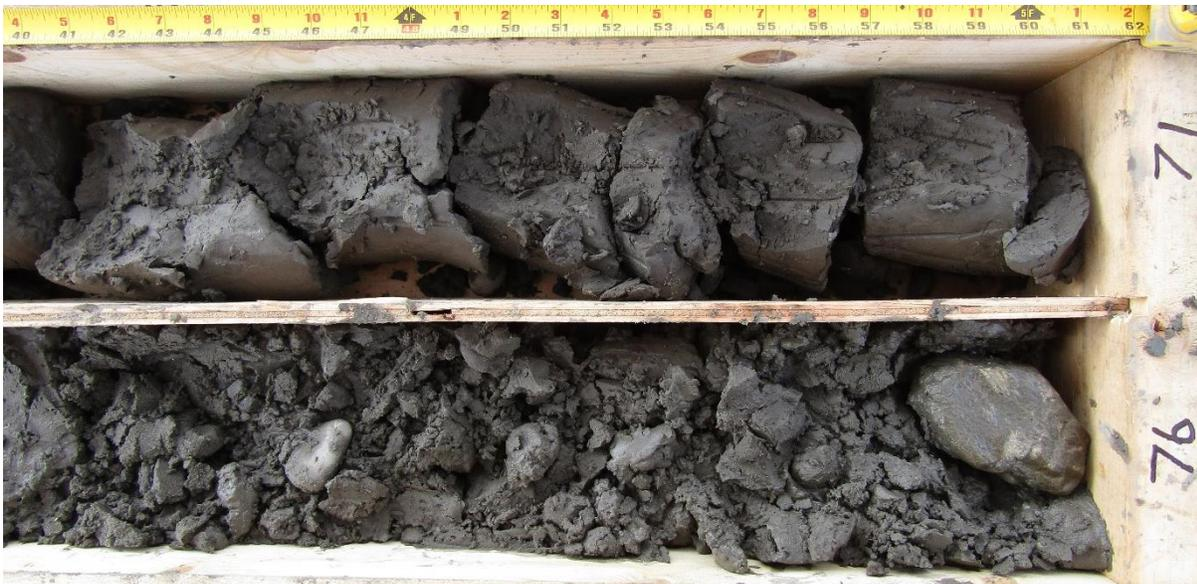
Figure 21. Massive, soft, grey silts at about 21.5 m (top box, 70-71 ft) overlying moist to wet, pebbly fine sands at about 23 m depth (bottom box, 74.5-76 ft) in sonic hole 10x
