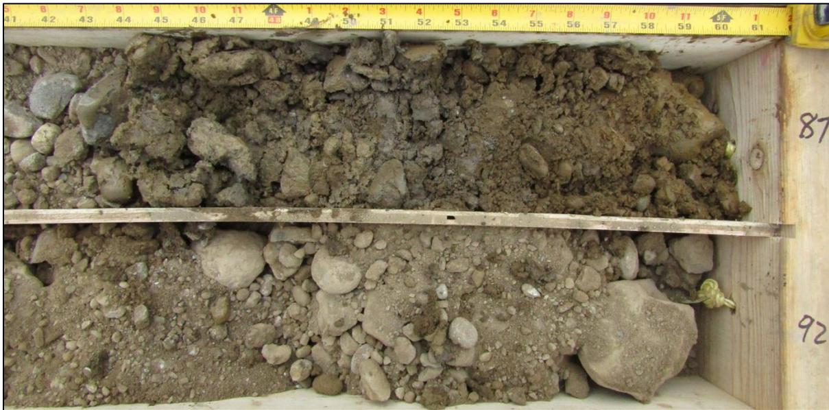
Figure 33. Interbedded pebble to cobble gravels at about 26-28 m depth (upper box 85.5-87 ft, lower box 90.5-92 ft) in sonic hole 13, interpreted to be glaciofluvial gravels of Cordilleran provenance
