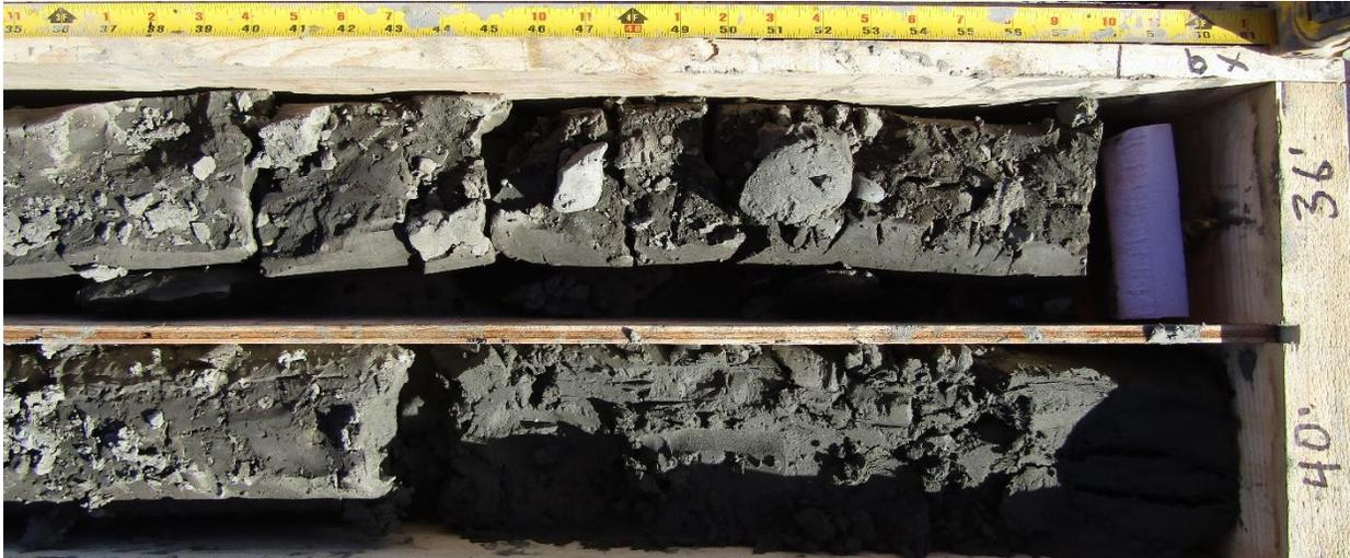
Figure 20. Massive, matrix-supported diamict in sharp contact with fine sands (contact is just left of center in the lower box); contact is at about 11.9 m (39 ft) at sonic drill hole 10x; scale in inches
