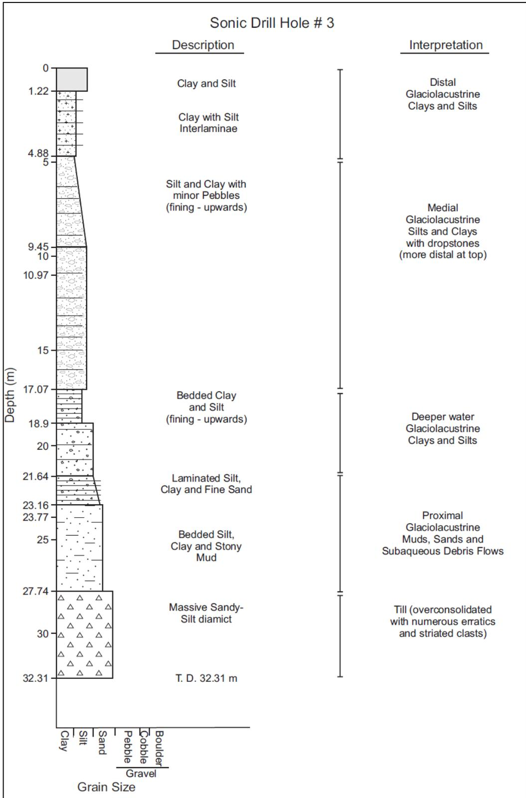
Figure 3. Stratigraphic log and interpretation of main units at sonic drill hole 3
