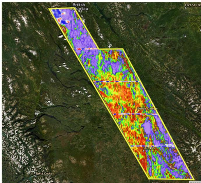
Undercover and Deep Geology from QUEST Electromagnetic and Gravity Data
