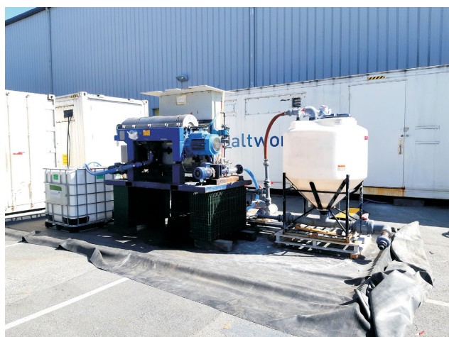
Figure 3. AirBreather pilot solids management subsystem showing centrifuge (left) and process tank (right).
