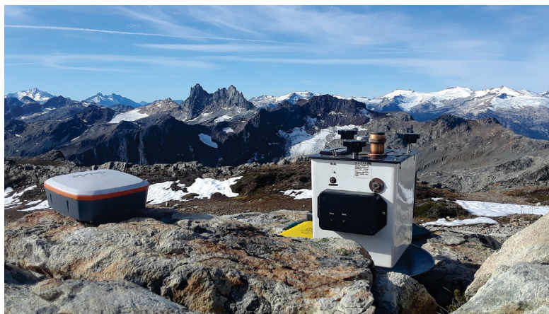
Figure 2. Gravity meter on the top of Mount Brandywine. Photo by A. Calahorrano-Di Patre.
