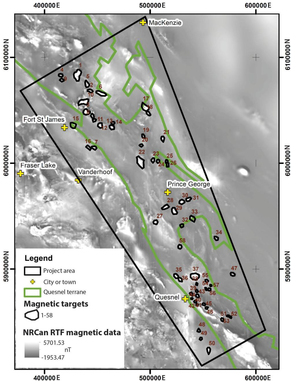
**Figure 3.** Magnetic targets selected for investigation (outlined in black; n = 58) superimposed on the Natural Resources Canada residual-total-field magnetic data grid (Natural Resources Canada, 2020). The Quesnel terrane is outlined in dark green, and the project area lies within the black quadrilateral. Abbreviation: nT, nanotesla.
