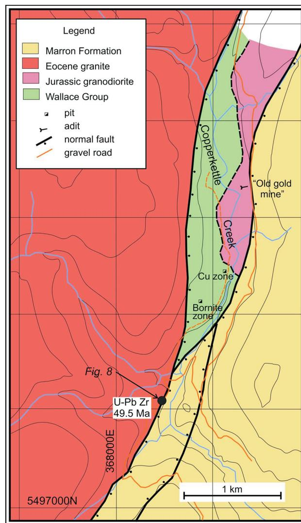
**Figure 7.** Geology of the western margin of the Rock Creek graben in the Boundary area, showing fault splays and location of chalcopyrite-galena-gold vein and skarn mineralization of the Copket property (location of the Eocene(?) dike, sample CV-294 and Figure 8 are also shown). Map modified from Whiting (1991) and Höy and DeFields (2017).
