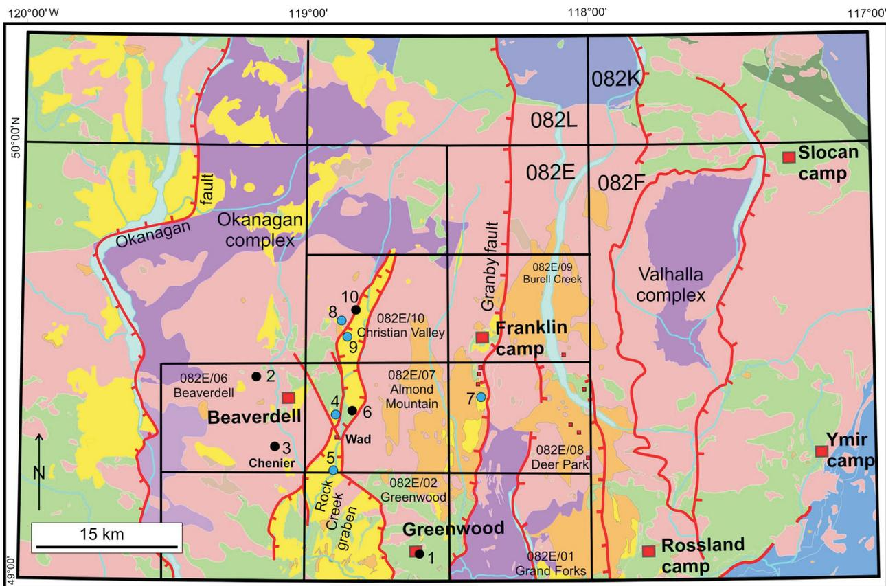
**Figure 1.** Regional terrane map of the Boundary area of southern British Columbia, showing location of major deposit camps, mineral occurrences discussed in this paper, and samples (numbered 1–10) collected for Ar/Ar and U-Pb dating.
