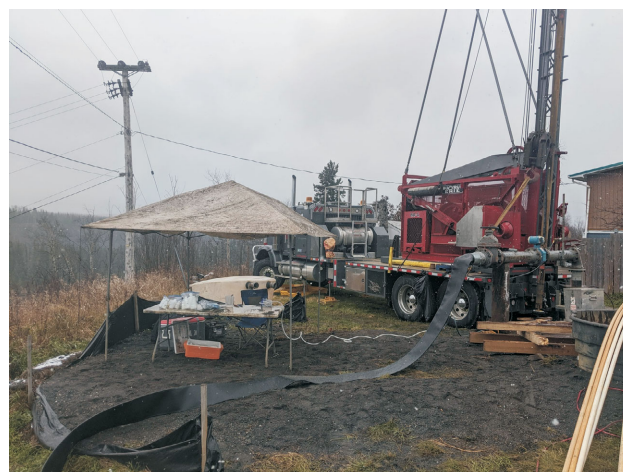
Figure 2. Sampling setup at one of the production wells during a constant-rate pumping test in November 2019, near Hudson's Hope, northeastern British Columbia.
