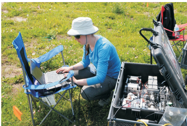
Figure 6. Operation of the miniRUEDI at Hudson's Hope Field Research Station.
