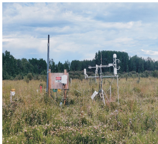
Figure 7. Eddy covariance system configuration at Hudson's Hope Field Research Station.
