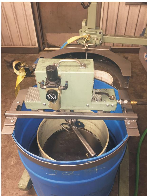
**Figure 4.** Roben Jig equipment used in this study.
