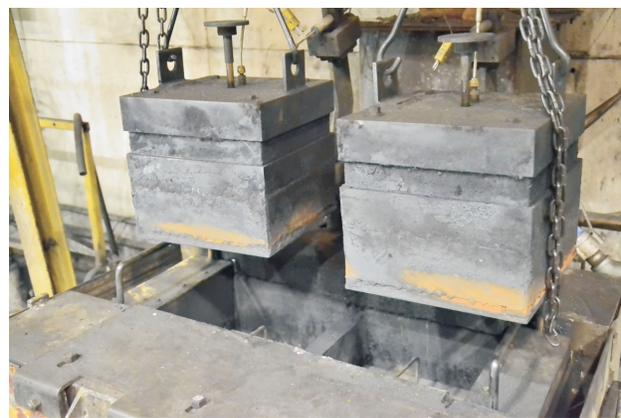
**Figure 7.** CanmetENERGY sole-heated oven (12 kg capacity) used in this study.
