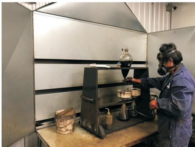
**Figure 3.** Operator working with organic liquids in a specially designed fume hood.
