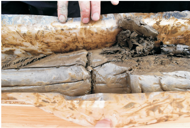
Figure 7. Sonic core composed of glacial clay/diamict, which dominates the upper portion of the Quaternary section throughout the Peace region, British Columbia.
