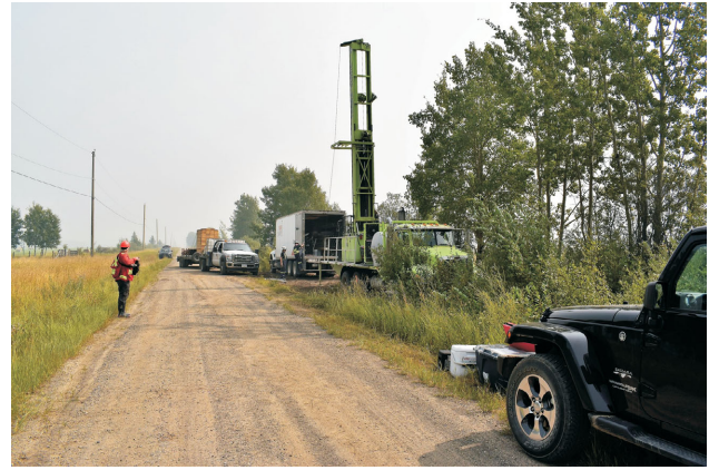
Figure 6. Sonic drilling in progress at Groundbirch field, Peace region, British Columbia.
