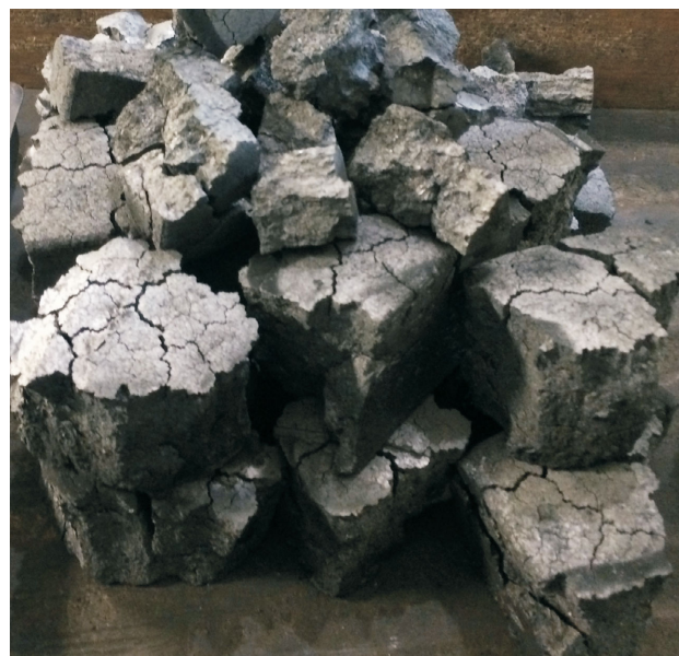
Figure 8. Coke made by carbonizing coal C, cleaned using the float-and-sink method, in the sole-heated oven.
