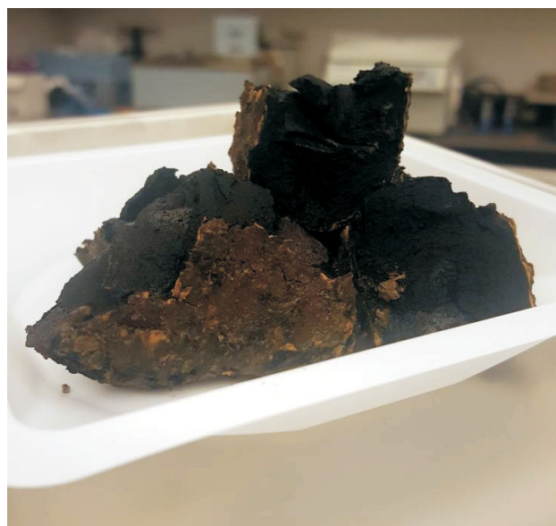
Figure 1. Residual from biological treatment of mine-impacted waters, showing evidence of Fe oxidation on the edges.
