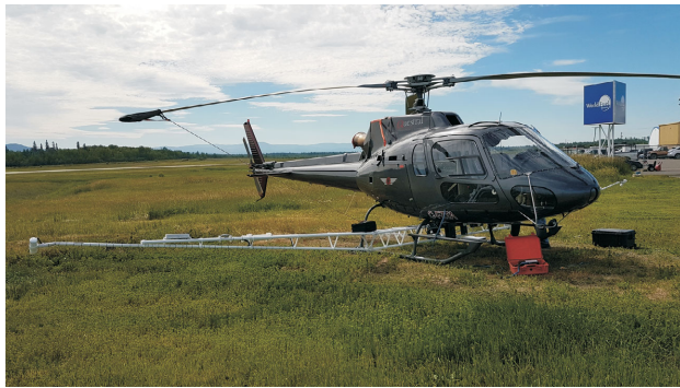
Figure 5. One of two helicopters used in flying the Search Phase III survey. The aircraft were fitted with booms to collect magnetic data using the proprietary Midas horizontal-gradient system of CGG Canada Services Ltd. Radiometric data were collected utilizing a Radiation Solutions Inc. RS-500 digital airborne gamma-ray spectrometer.
