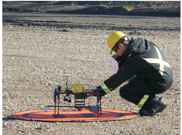
Figure 7. Deployment of NASA Jet Propulsion Laboratory's open-path laser spectrometer mounted on InDro Robotics Inc.'s small unmanned aerial vehicle.
