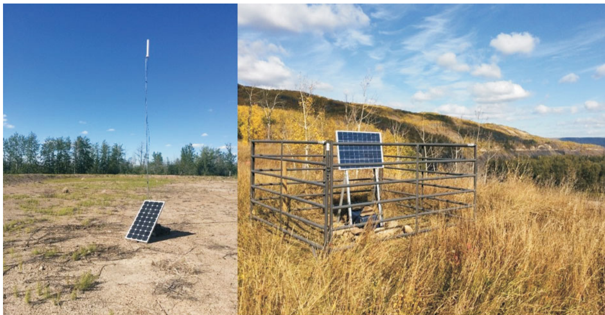
Figure 2. Field setup of a temporary (right) and a long-term station (left) used to monitor the Montney Formation.
