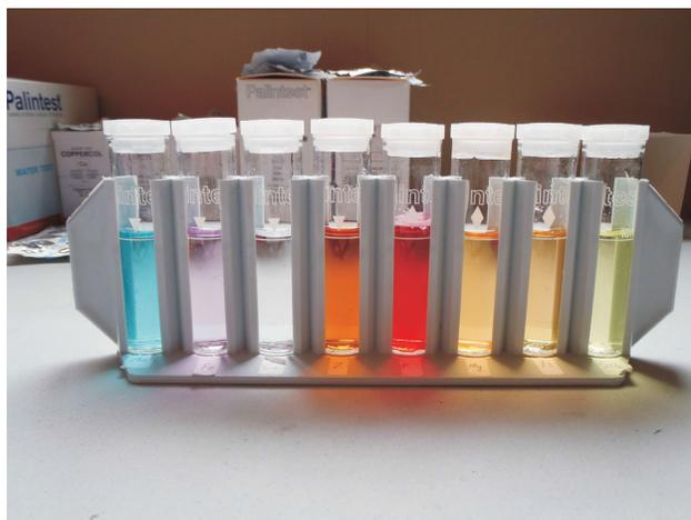
**Figure 3.** Collection of reagents ready for photometer testing. Note the clear Cu test (third from the left) that could be susceptible to turbidity interference, which occurs when the photometer records a false concentration because the solution is darker due to turbidity.
