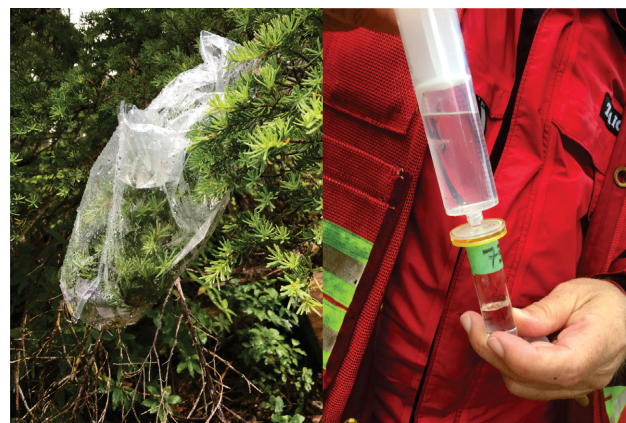
Figure 5. Collection of transpired fluid (left) and filtration of fluid into glass vial (right).
