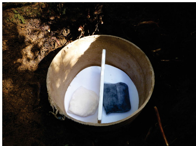
Figure 4. Partly installed ion collector showing sachets of activated carbon (right) and ion-exchange resin (left) separated by a ceramic partition. Cardboard tube is 18 cm in diameter.
