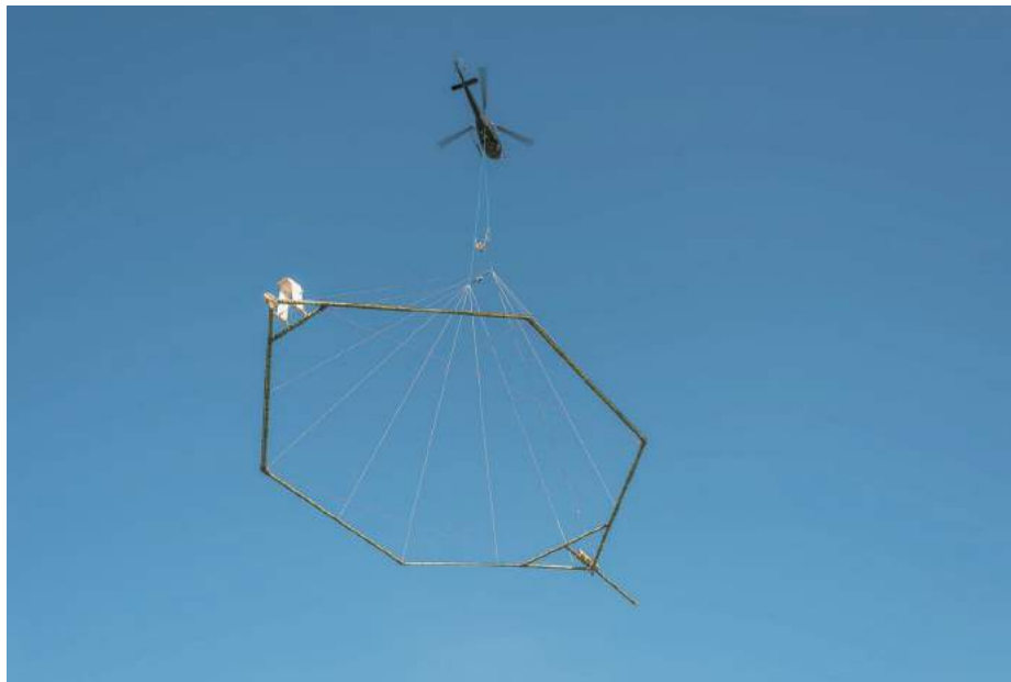
Figure 2: The SkyTEM312 Fast system in operation.
