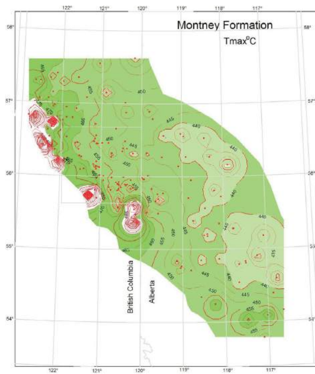
Figure 5. Regional thermal maturity of the Montney Formation, northeastern British Columbia, based on selective T_{max} values from Rock-Eval-type analyses. The lighter green corresponds to the early stage of the oil window and the darker green, to the last stage.
