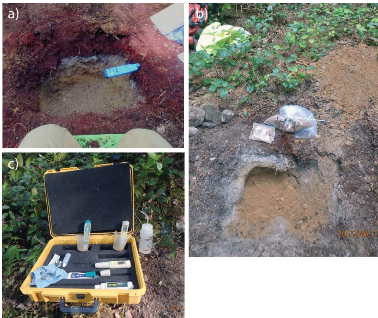
Figure 8. Sampling procedure: a) the direct soil measurement of electrical conductivity; b) a completed sample with the pit showing a portion of the B horizon removed; c) slurry-based measurements in the field, including free chlorine on the left and pH on the right.
