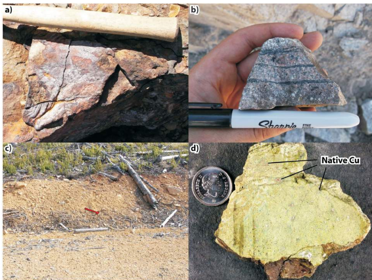
Figure 4: a) Gossanous Skeena Group conglomerate with apparent flow-top texture in bottom left corner. Sample collection site for 14JA111A; b) sheeted magnetite-pyrite veinlets with K-feldspar alteration haloes at the Havana showing; c) gossanous till composed predominantly of quartz-sericite-pyrite-altered andesite at the Havana showing, rock hammer for scale highlighted in red; d) native Cu in epidote-calcite-quartz vein float at the Liesegang showing.
