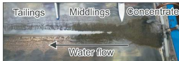
Figure 5. View of the surface of the Mozley C800 laboratory mineral separator table and sample material after a completed run. Concentrate, middlings and tailings are separated based on pattern and colour of the material stream.
