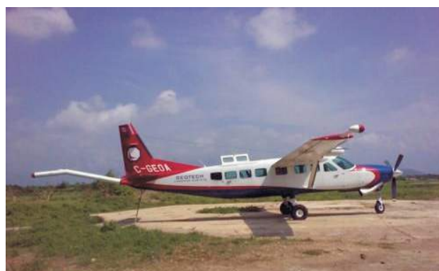
Figure 2. Aeroquest Airborne Ltd. Cessna Caravan C208B used to fly the TREK survey over the Interior Plateau region of south-central British Columbia. Photo courtesy of Aeroquest Airborne Ltd.
