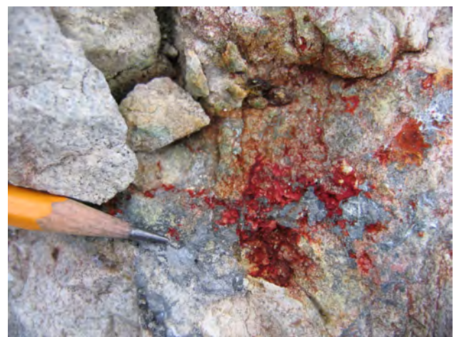
Figure 17. Typical bright red reaction of Zinc Zap solution in a zinc-rich exposure, east-central British Columbia.
