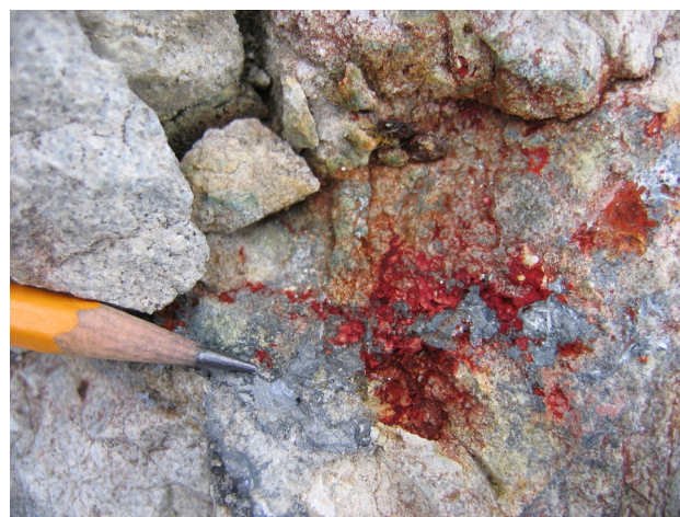
Figure 17. Typical bright red reaction of Zinc Zap solution in a zinc-rich exposure, east-central British Columbia.
