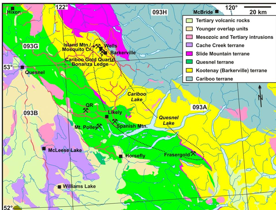
**Figure 1.** Regional geology of the study area in east-central British Columbia, showing locations of the Cariboo gold district (dotted black line), significant known lode-gold and copper-gold deposits (crossed rock hammer symbols) and significant placer streams (red lines).
