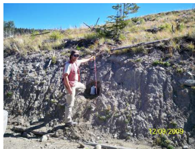
Figure 6. A typical roadcut basal till sample site, southern British Columbia.
