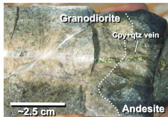
Figure 12. Quartz-chalcopyrite vein with a bleached, K-feldspar-bearing alteration selvage crosscutting andesitic and granodioritic rocks from the Main zone of the Huckleberry copper-molybdenum deposit, central British Columbia.
