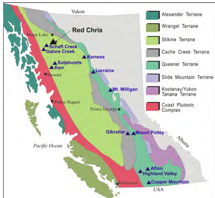
Figure 1. Major tectonic terranes and associated Mesozoic porphyry deposits of the Canadian Cordillera in British Columbia.
