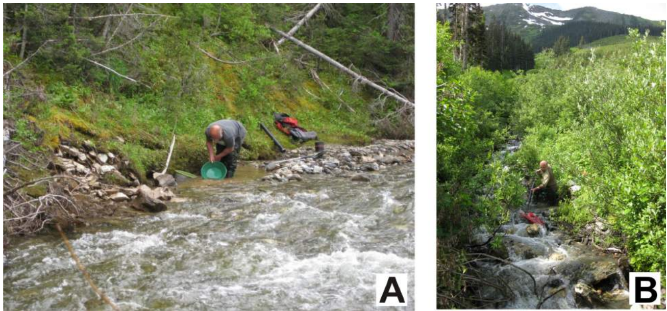
Figure 2. Collecting placer-gold samples in east-central British Columbia, using A) panning methods and B) a portable test sluice and hand pump.
