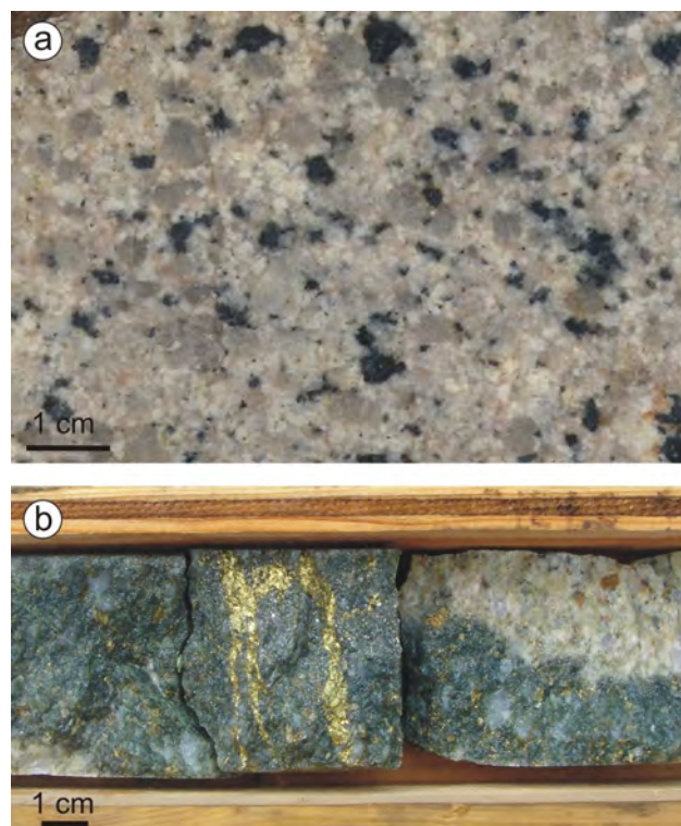
Figure 2. Examples of hostrock and alteration from the Alwin mine, Highland Valley, south-central British Columbia: a) sample of fresh Bethsaida granodiorite, the main hostrock to mineralization, with characteristic large, rounded quartz phenocrysts and biotite books; b) intense green mica alteration and associated chalcopyrite mineralization overprinting the Bethsaida granodiorite.
