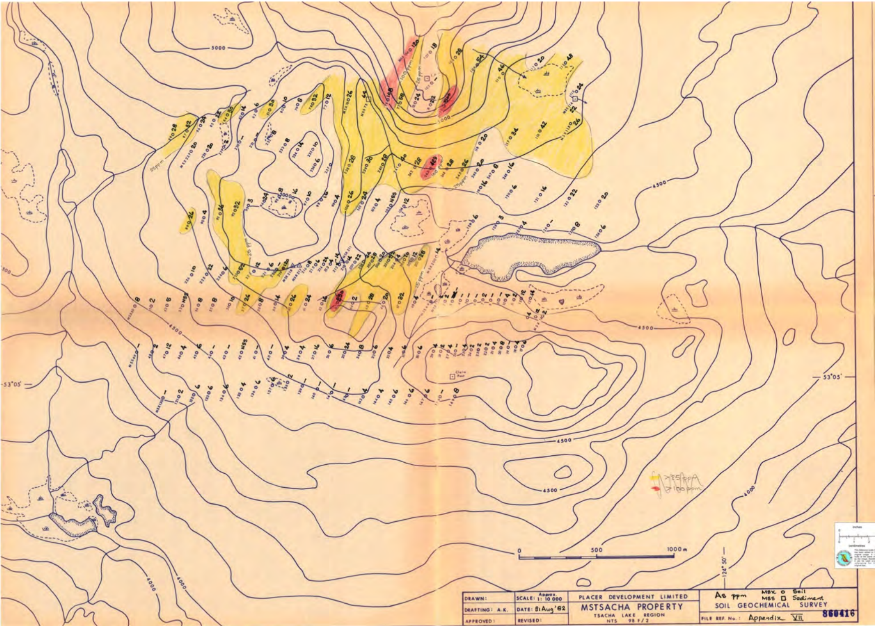
Figure 4. Soil and sediment geochemical survey map showing As sample values and contours, Ram occurrence, central British Columbia (Placer Development Limited, 1982).
