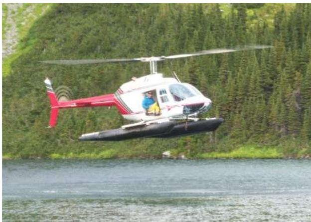
**Figure 5.** Interior Helicopter Ltd.'s helicopter equipped with floats, northern Nechako Plateau, central British Columbia.
