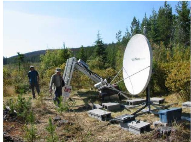
**Figure 3.** Photograph of Nechako seismic station RAMB, showing the typical station layout, with solar panels and a satellite dish (seismic vault is not visible).
