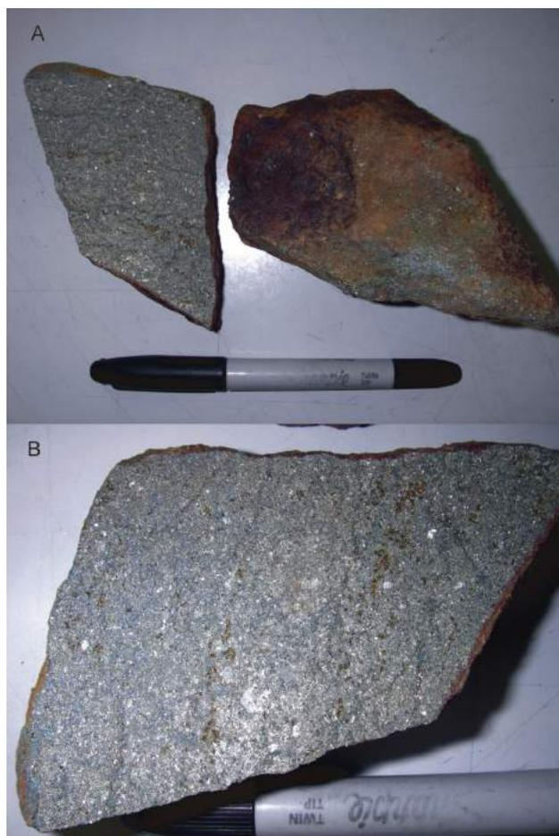
**Figure 4.** New massive sulphide mineralization discovered on the Westridge Resources Inc. mineral tenure in the Breen Lake area: **A)** medium- to coarse-grained massive pyrite with interstitial chalcopyrite and trace sphalerite; **B)** close-up of massive sulphide mineralization.
