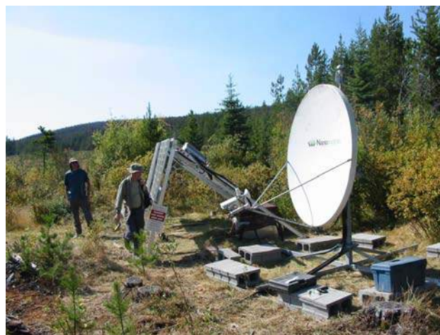
Figure 3. Photograph of Nechako seismic station RAMB, showing the typical station layout, with solar panels and a satellite dish (seismic vault is not visible).
